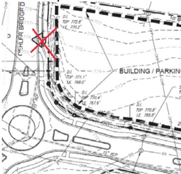
4. The petitioner should revise the site plan and conditional note(s) to extend the median on the southern side of Johnston Oehler Road to create the restriction needed for a RI/RO.
