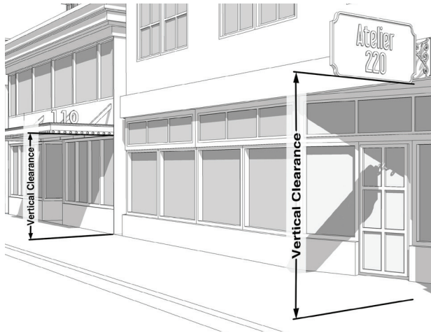
Measurement of Vertical Clearance
