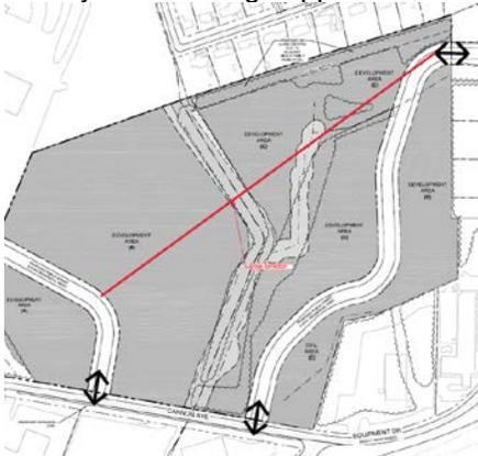
6. The petitioner should revise the site plan and conditional note(s) to realign the road extension to sugar creek so that the R/W completely abuts the property line as shown below. The realignment will provide access private/public drive to the parcels along West Sugar Creek Road, and reduce the number of driveways on Sugar Creek Road.
