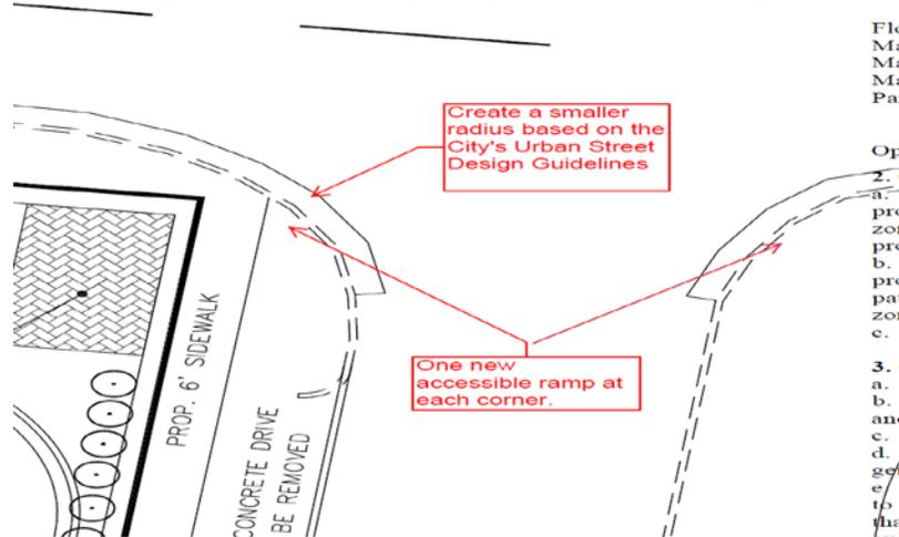
7. The petitioner should revise the site plan and conditional note(s) to create a smaller curb radius on the corner at Iris and Central.
