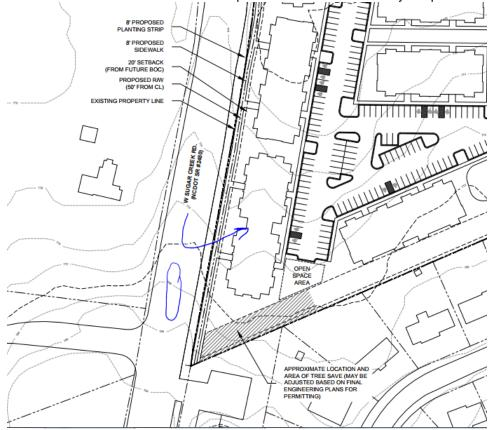
5. The petitioner should revise the site plan and conditional note(s) to revise the drive aisle shown below to allow permanent public access, use a form consistent with a public street section, and create a stub for future connection and cross access from adjacent parcels.
