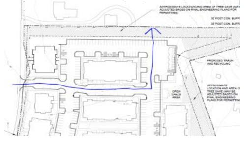
6. The petitioner should revise the site plan and conditional note(s) to remove the on-street parking shown in the first segment of the drive aisle connection to Sugar Creek.
