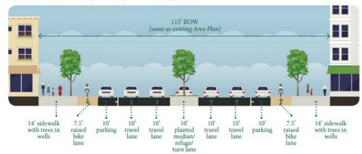
Figure 16: South Boulevard Segment 2 Proposed Section (Near term)
