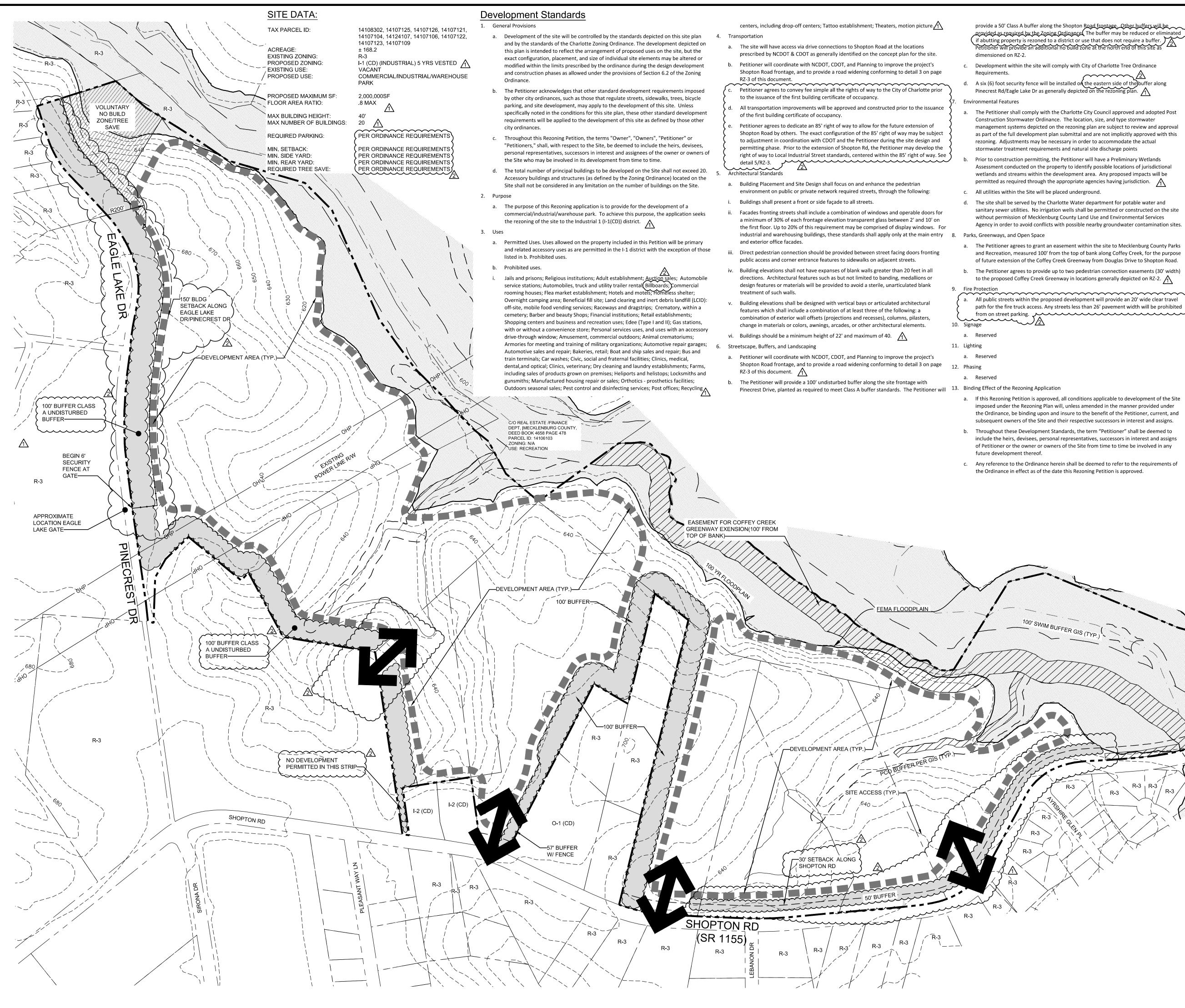
Fire Protection a. All public streets within the proposed development will provide an 20' wide clear travel path for the fire truck access. Any streets less than 26' pavement width will be prohibited from on street parking.
