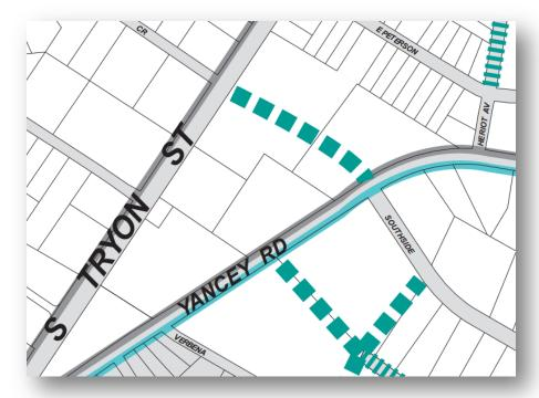
2. The petitioner should revise the site plan along S. Tryon to match the Scaleybark Transit Station Area Plan. The future back of curb on S. Tryon St is 38' from the centerline of the roadway. The setback on S. Tryon needs to be measured from this future location. Petitioner should dimension 38' from centerline to future back of curb and required setback from future back of curb to future building.
