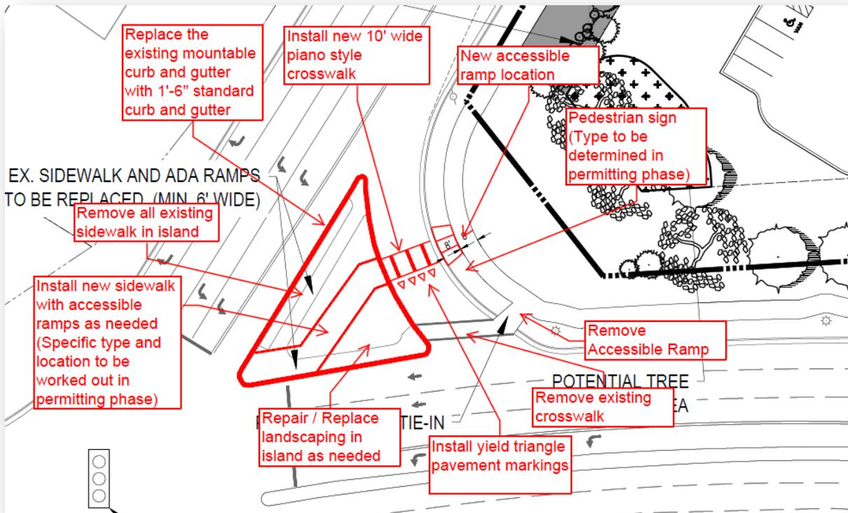
2. CDOT requests that the petitioner install two accessible ramps at the existing right in access on of Tyvola Rd. See below:
