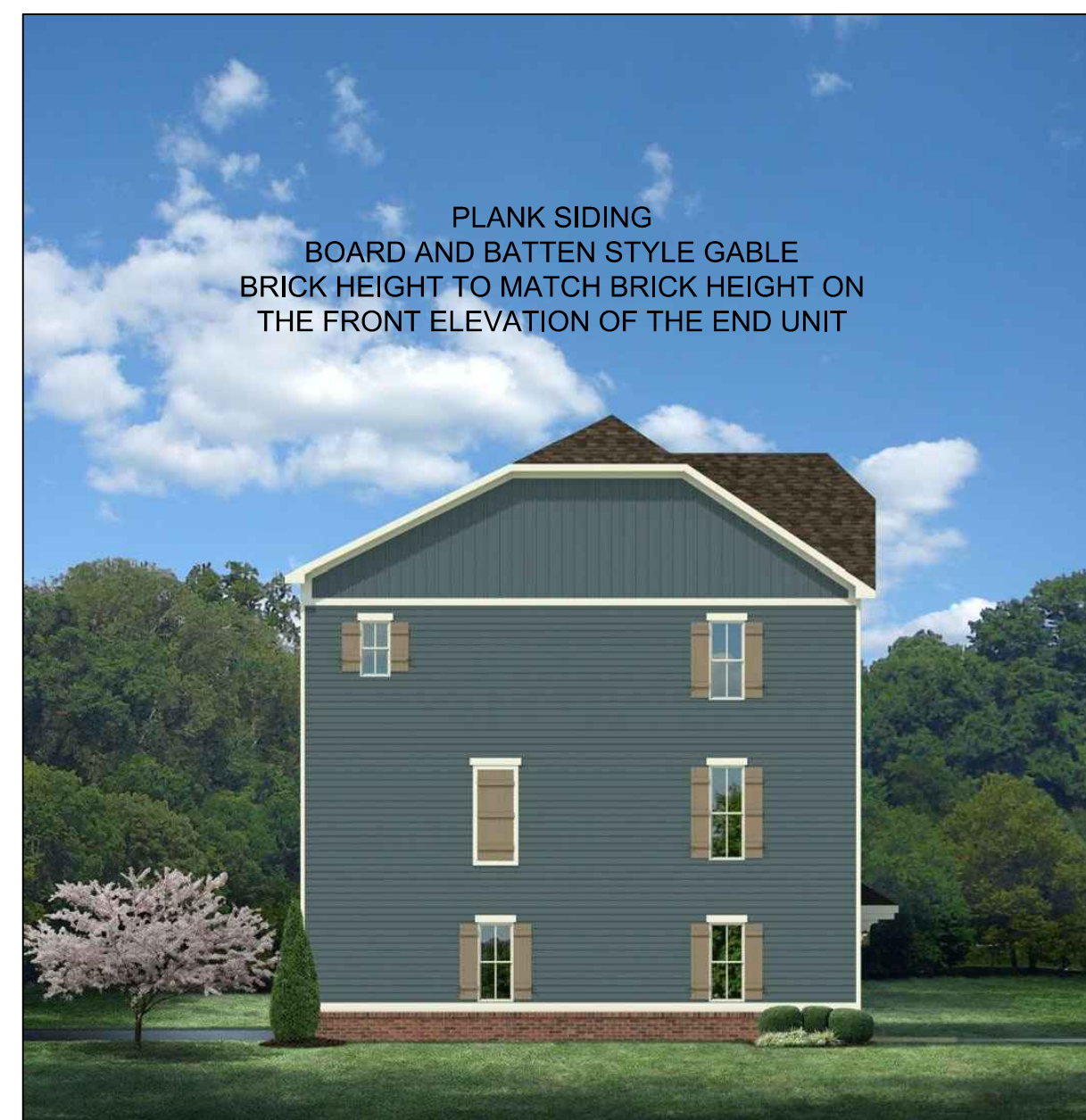
GABLE END ELEVATION - THREE STORY FRONT
