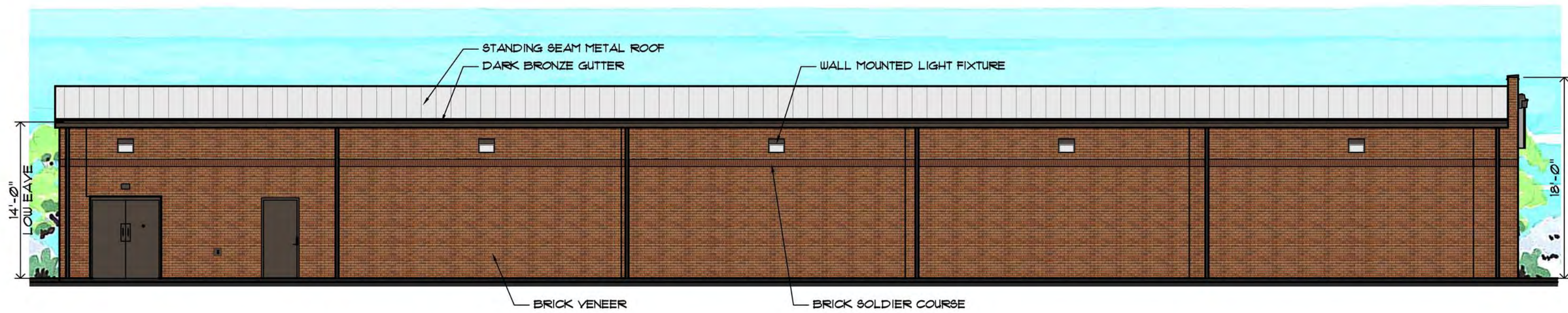
3 LEFT SIDE ELEVATION A2.B 1/8"=1'-0"
