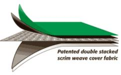
patented weave that is lightweight yet exceptionally strong. Covers are also UVI treated and weather resistant for long-lasting use, and flame retardant material is available. Nova-Shield II™ with ArmorKote<sup>™</sup> covers have a 15 year warranty. ClearSpan's pre-engineered truss arch structures meet all wind and snow load regulations.
