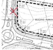
4. The petitioner should revise the site plan and conditional note(s) to extend the median on the southern side of Johnston Oehler Road access to create the restriction needed for a RI/RO.
