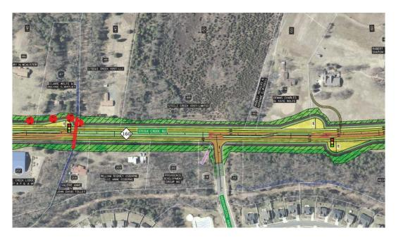
b. Sledge Road: Location of curb and gutter should be moved to 27 feet from existing centerline, to accommodate for the Comprehensive Transportation Plan's recommended thoroughfare improvements for a future 2-way divided buffered bike lane cross section. The site plan should show the curb and gutter labeled and dimensioned from the centerline for each road.
