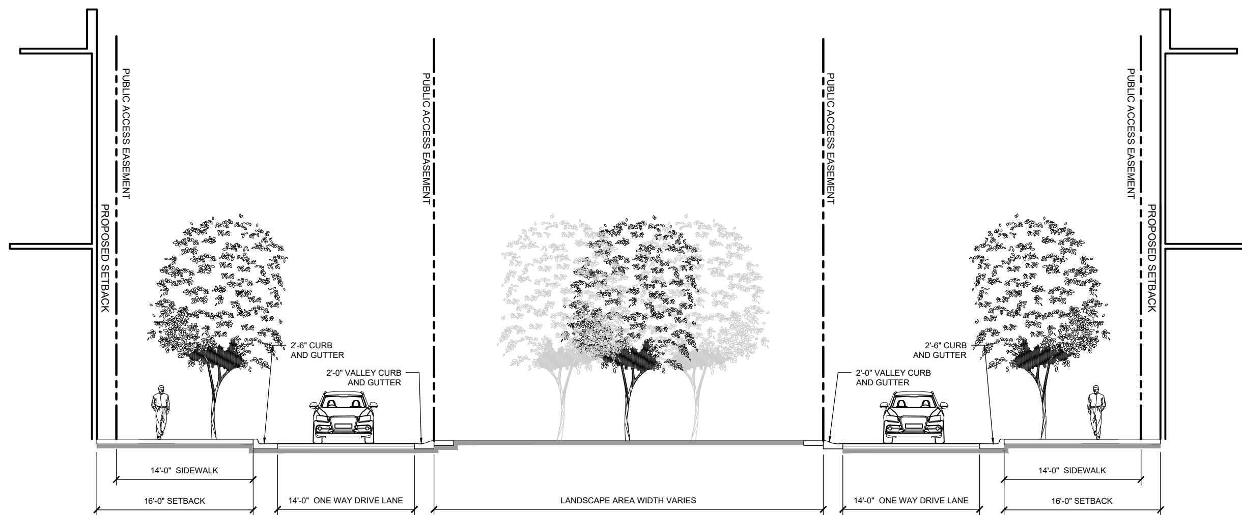
MAIN STREET AT PARK CROSS-SECTION SECTION C-C SCALE: 1" = 10'-0"
