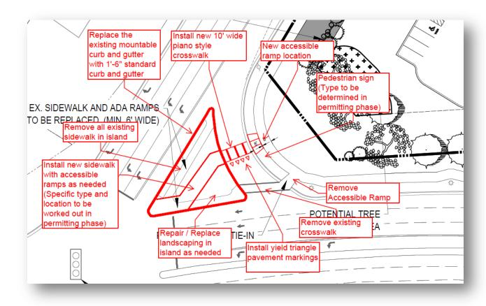
2. CDOT requests that the petitioner install two accessible ramps at the existing right in access on of Tyvola Rd. See below:
