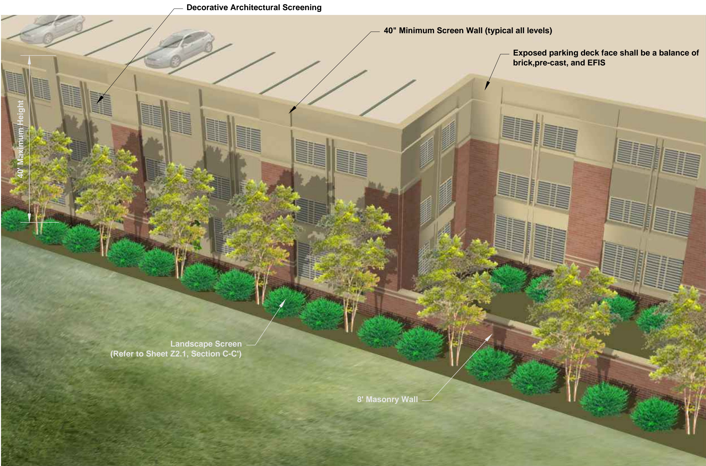
C - STRUCTURED PARKING DECK ELEVATION ALONG SOUTH PROPERTY LINE
