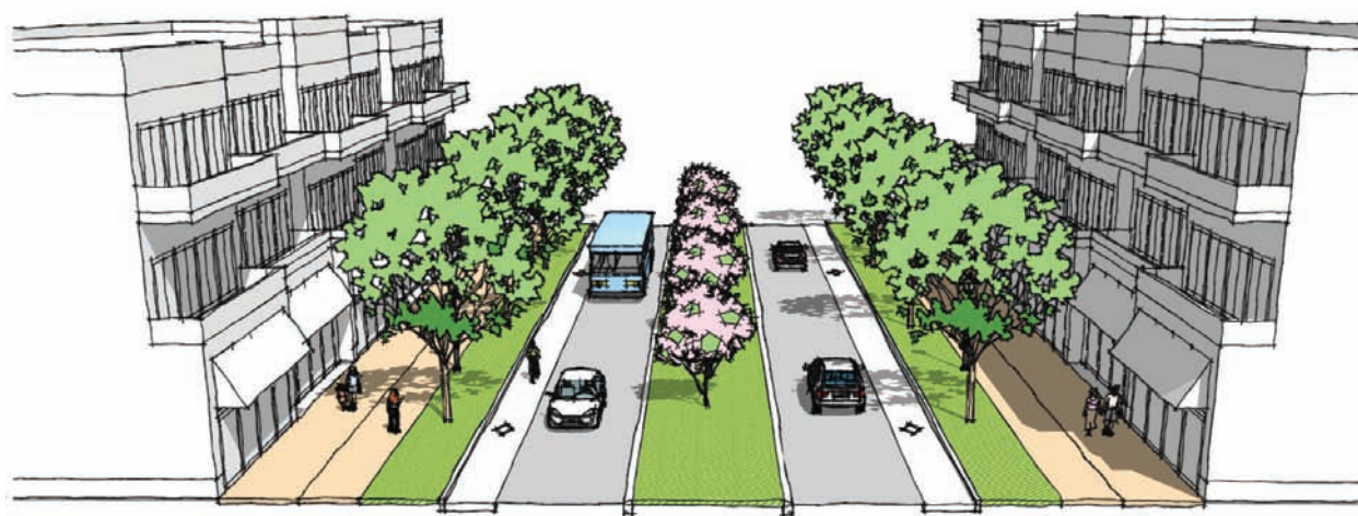
Figure 10 3-Lane Avenue (w/o parking) Cross-Section
