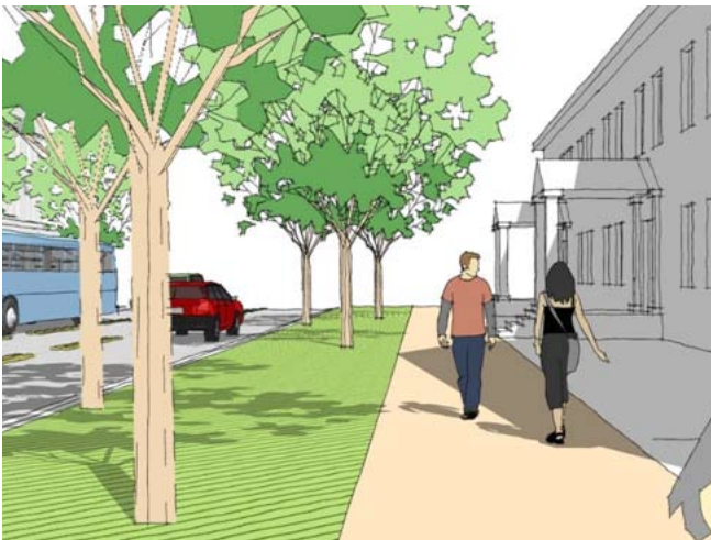
In areas where ground floor residential uses are prevalent, a 13' wide planting strip and 8' sidewalk are recommended. A secondary row of street trees can supplement the street's existing mature trees. Landscaped front yards may separate the buildings from the back of the sidewalk.
