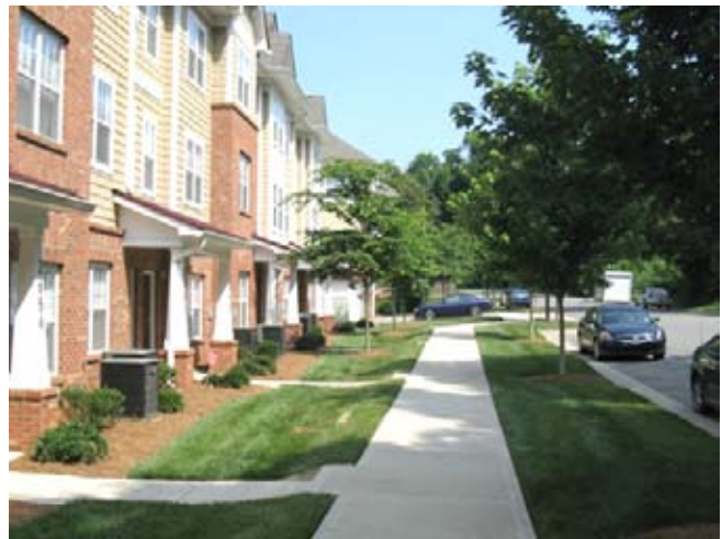
This residential development on Weddington Avenue, a good example of cross-section B2 , features a wide planting strip with trees. This area also has recessed on-street parking. Landscaped front yards separate the dwelling units from the public sidewalk, connected with individual walkways.
