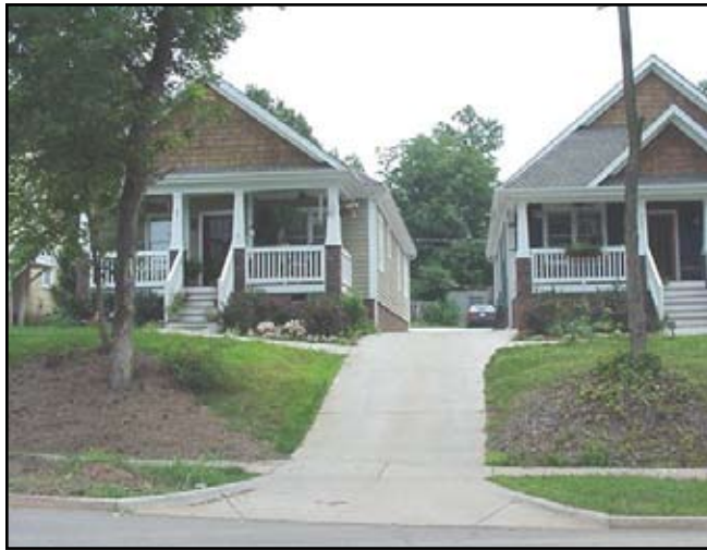
Shared driveways minimize pedestrian obstructions and impervious surface
