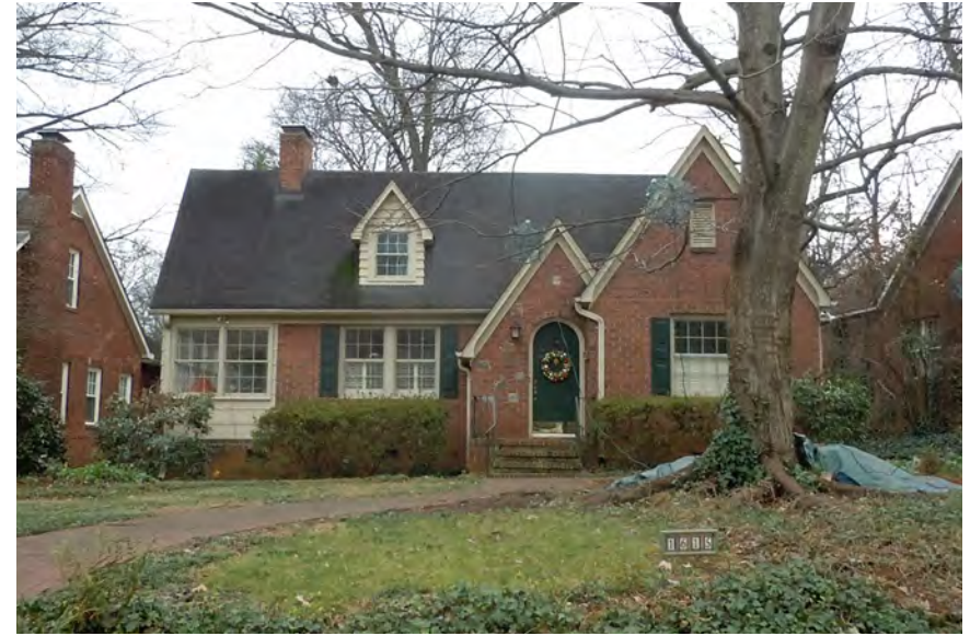
This English Cottage style has an entry gable that attaches to the larger end gable. Note the round arch front door and steeply pitched roof.
