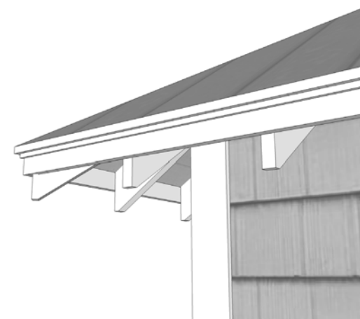
Craftsman styled trim details may include corner boards and exposed rafter ends.
