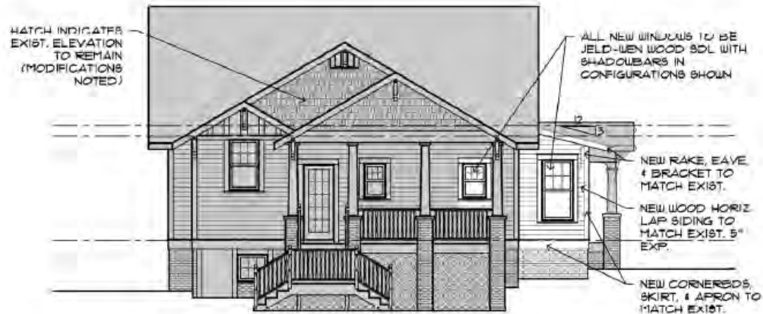
2 REAR ELEVATION (SOUTH) - PROPOSED A22 SCALE: 1/8"=1'-0"
