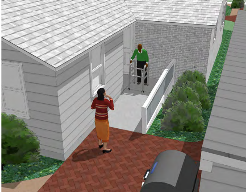
This entry ramp is conveniently placed to lead from the side driveway to a nearby secondary entrance to the house.
