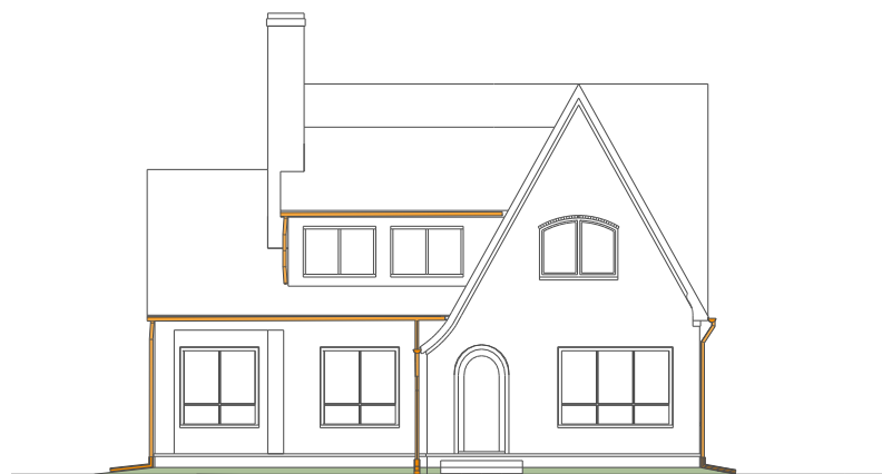
Well placed and properly installed gutters and downspouts are essential for protection from moisture infiltration.
