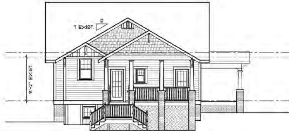
1 REAR ELEVATION (SOUTH) - EXISTING A22 SCALE: 1/8"=1'-0"
