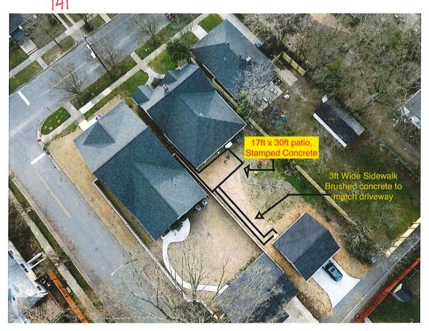
The dimensions selected were to follow historic guidelines in not allowing greater than 50% of the backyard to be of impermeable material with the recent garage/driveway construction. Neither the walkway or the patio will be visible from the street. The backyard is fenced in.
