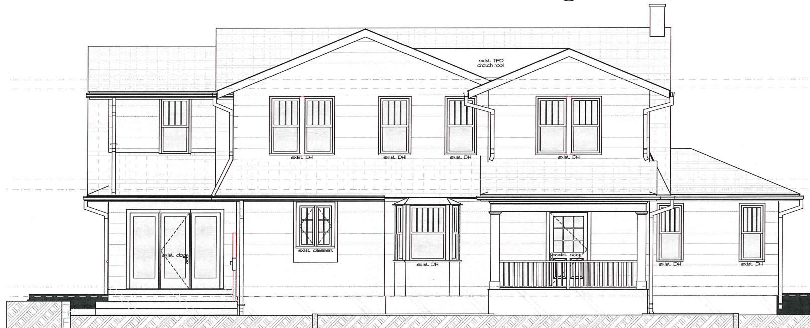
1 AS-BUILT REAR ELEVATION SCALE: 1/4" = 1'-0"
