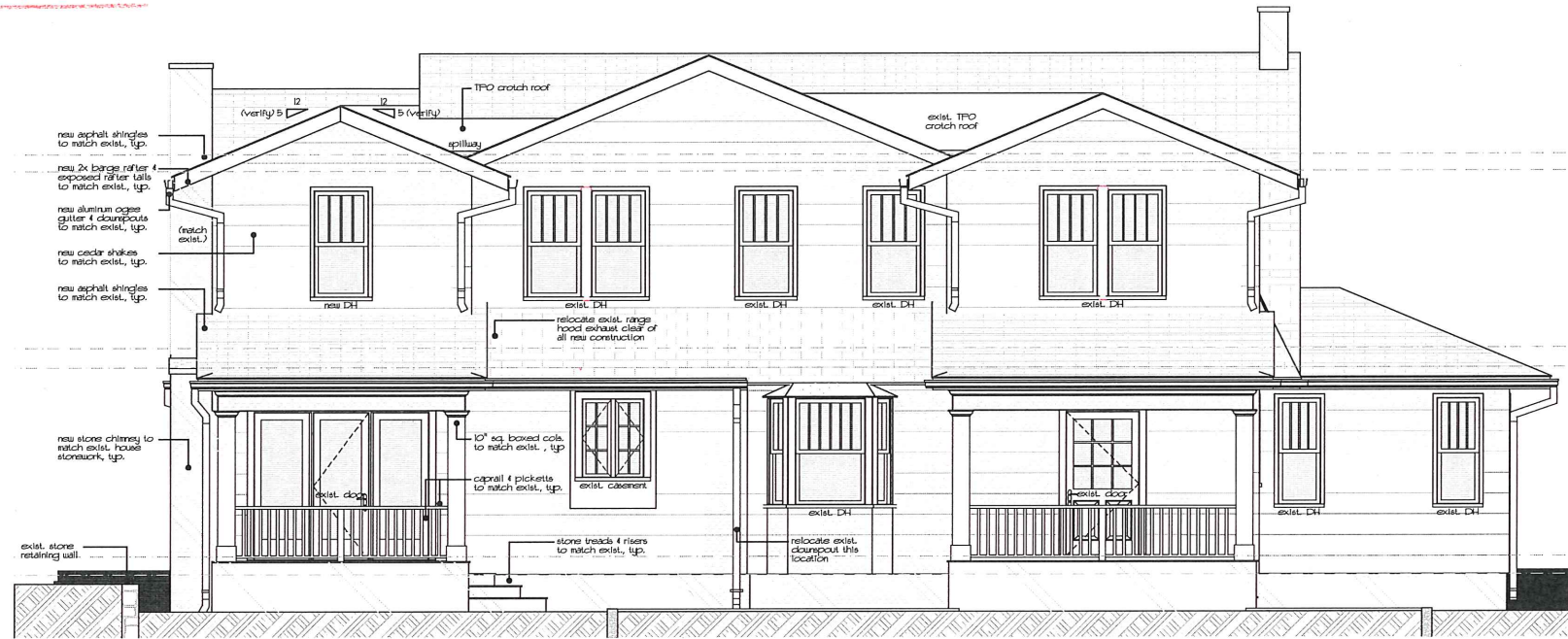
3 PROPOSED REAR ELEVATION SCALE: 1/4" = 1'-0"
