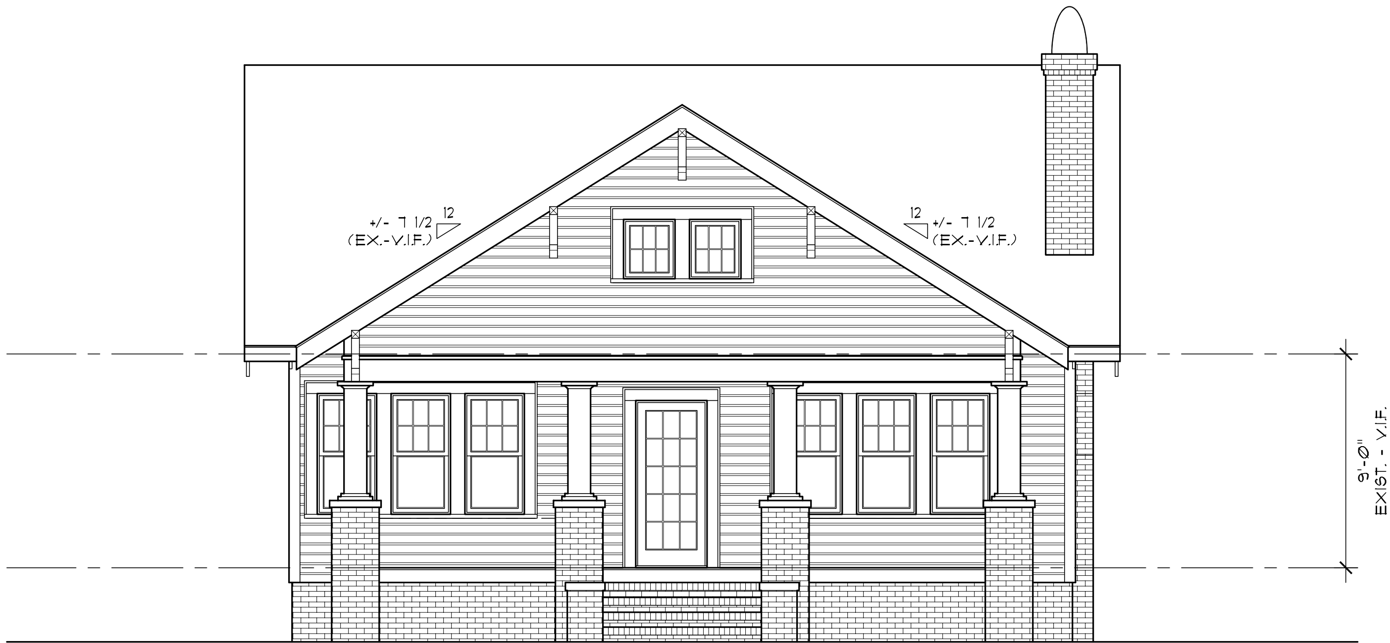
RESTORED / REPAIRED FRONT (NORTHEAST) ELEVATION - EAST KINGSTON AVENUE 1 A2.0 SCALE: 1/8"=1'-0"
