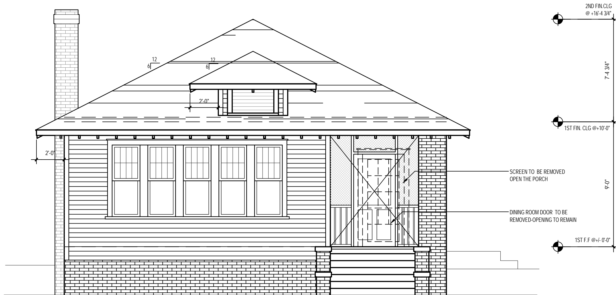
② EXISTING FRONT ELEVATION 1/4" = 1'-0"
