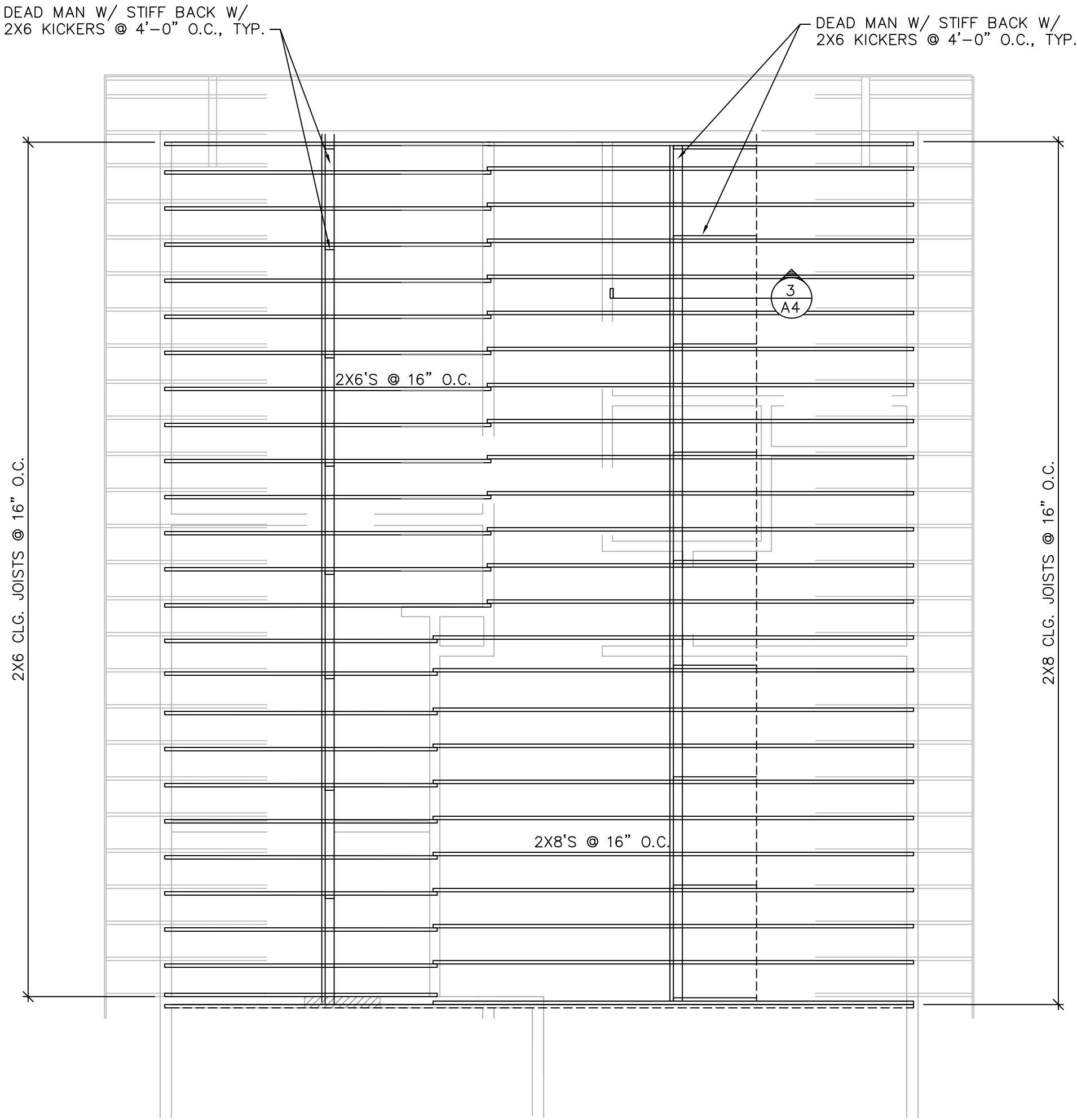
2 A4 CEILING FRAMING PLAN 1/4"=1'-0"
