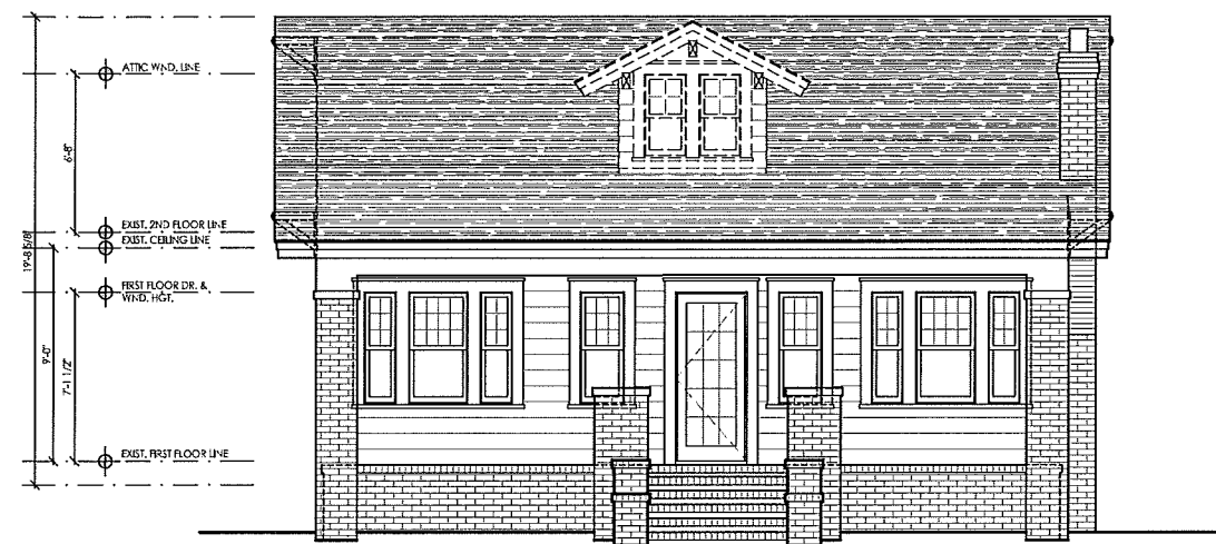
1A EXISTING FRONT ELEVATION 2.1 Scale: 1/4" = 1'-0"
