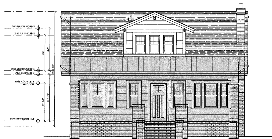
1B NEW FRONT ELEVATION 2.1 Scale: 1/4" = 1'-0"
