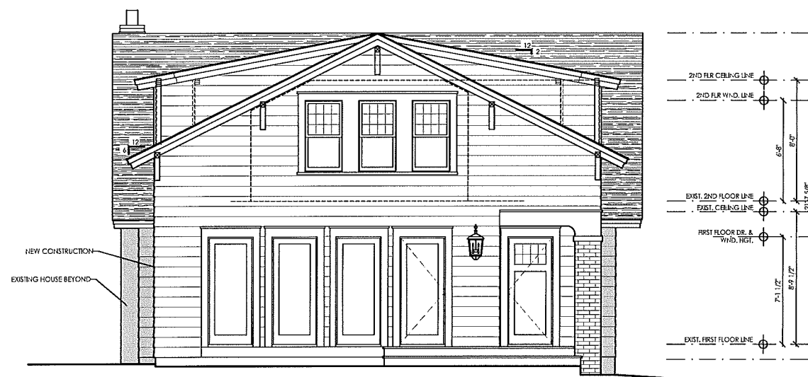
2B NEW REAR ELEVATION 2.1 Scale: 1/4" = 1'-0"
