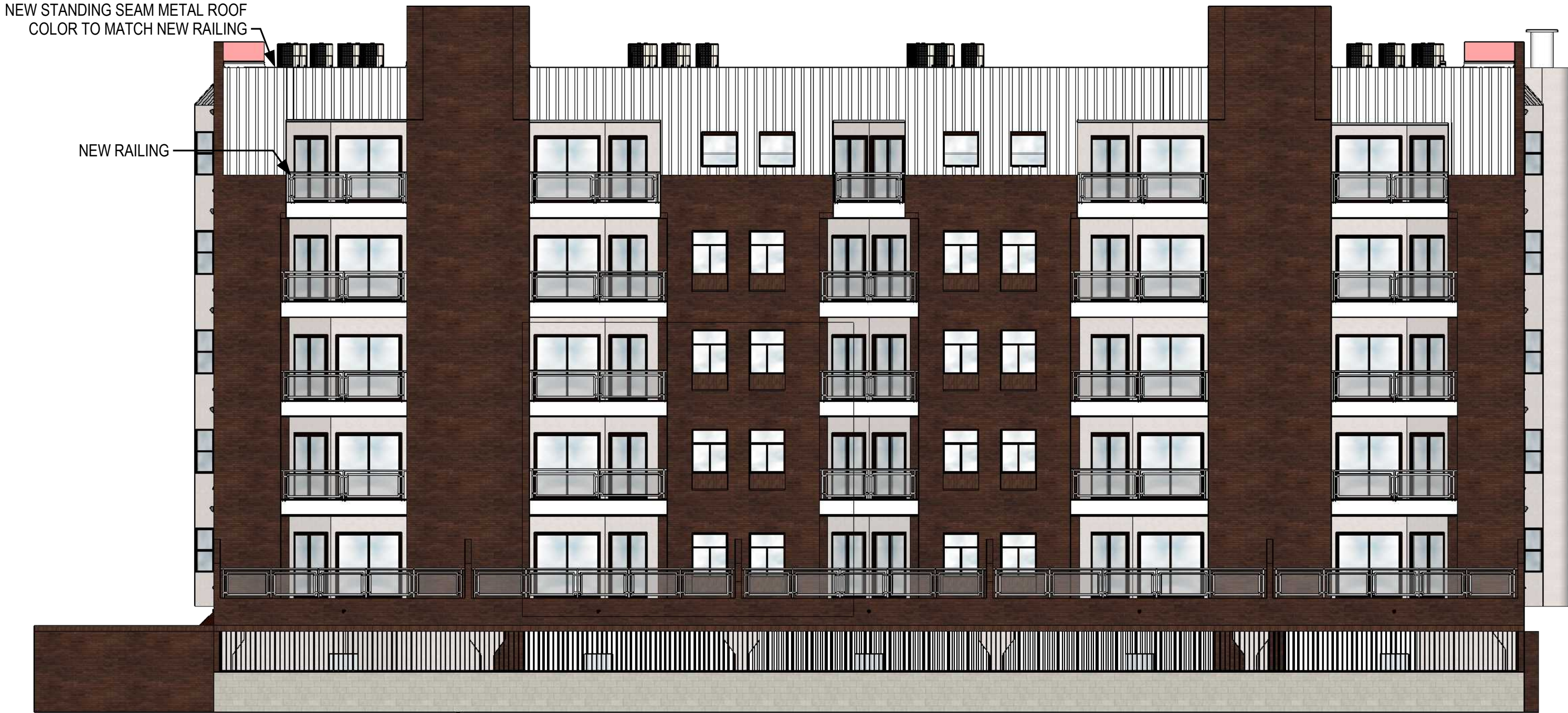
EAST ELEVATION - PROPOSED RAILING : PRIVACY RAILS
