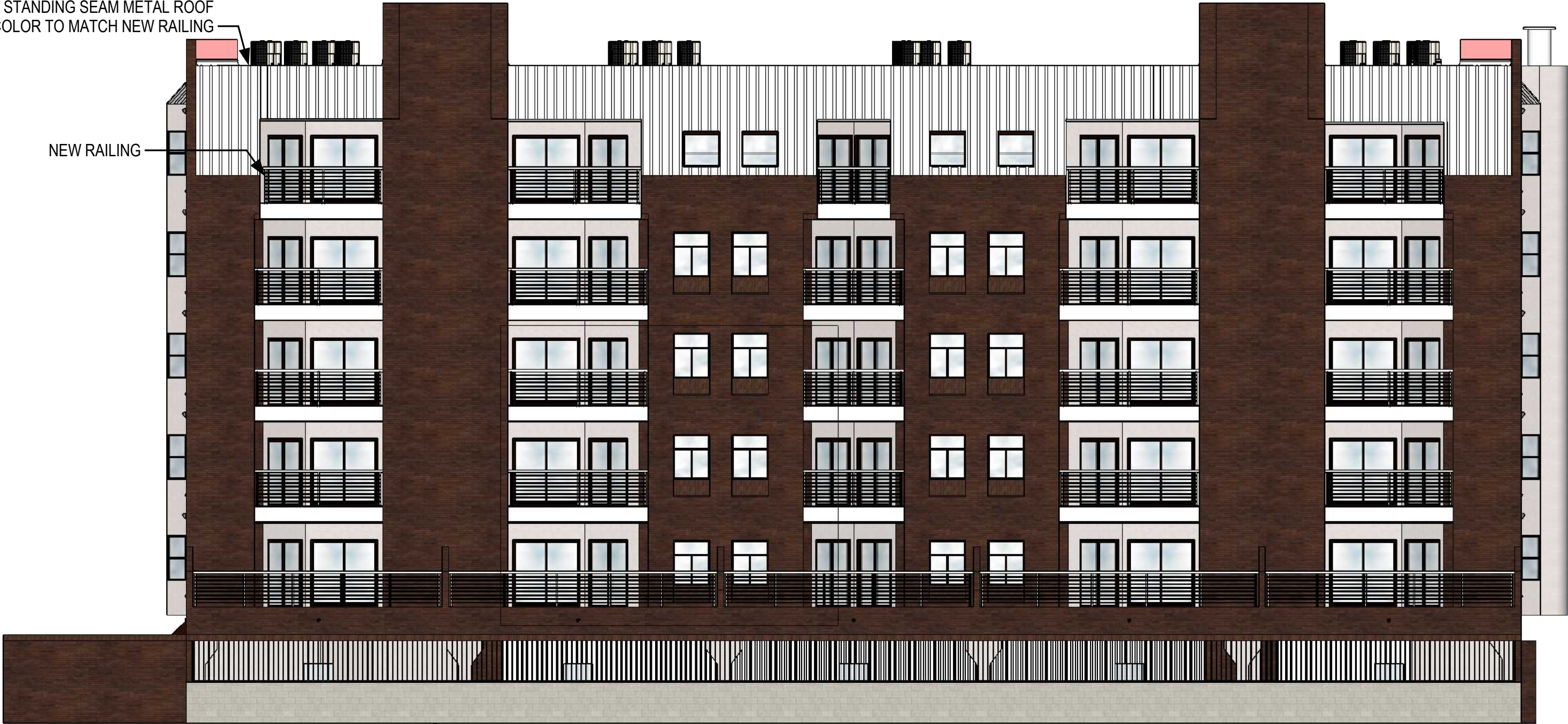
EAST ELEVATION - PROPOSED RAILING : HORIZONTAL RAILS
