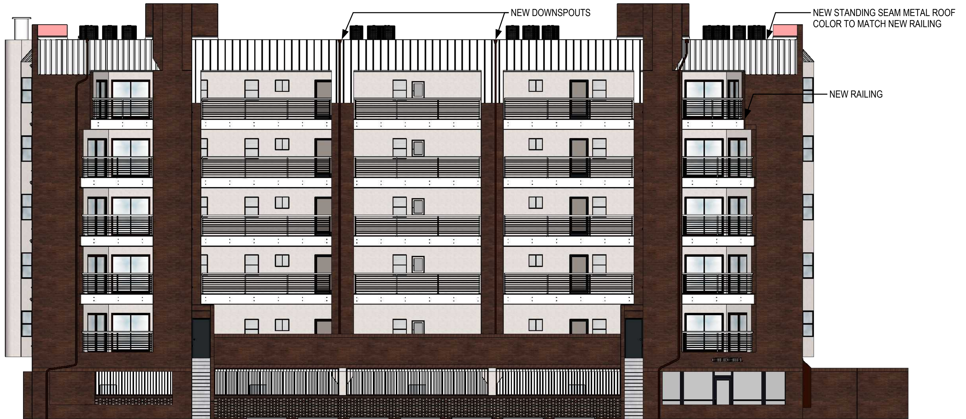
WEST ELEVATION - PROPOSED RAILING : HORIZONTAL RAILS
