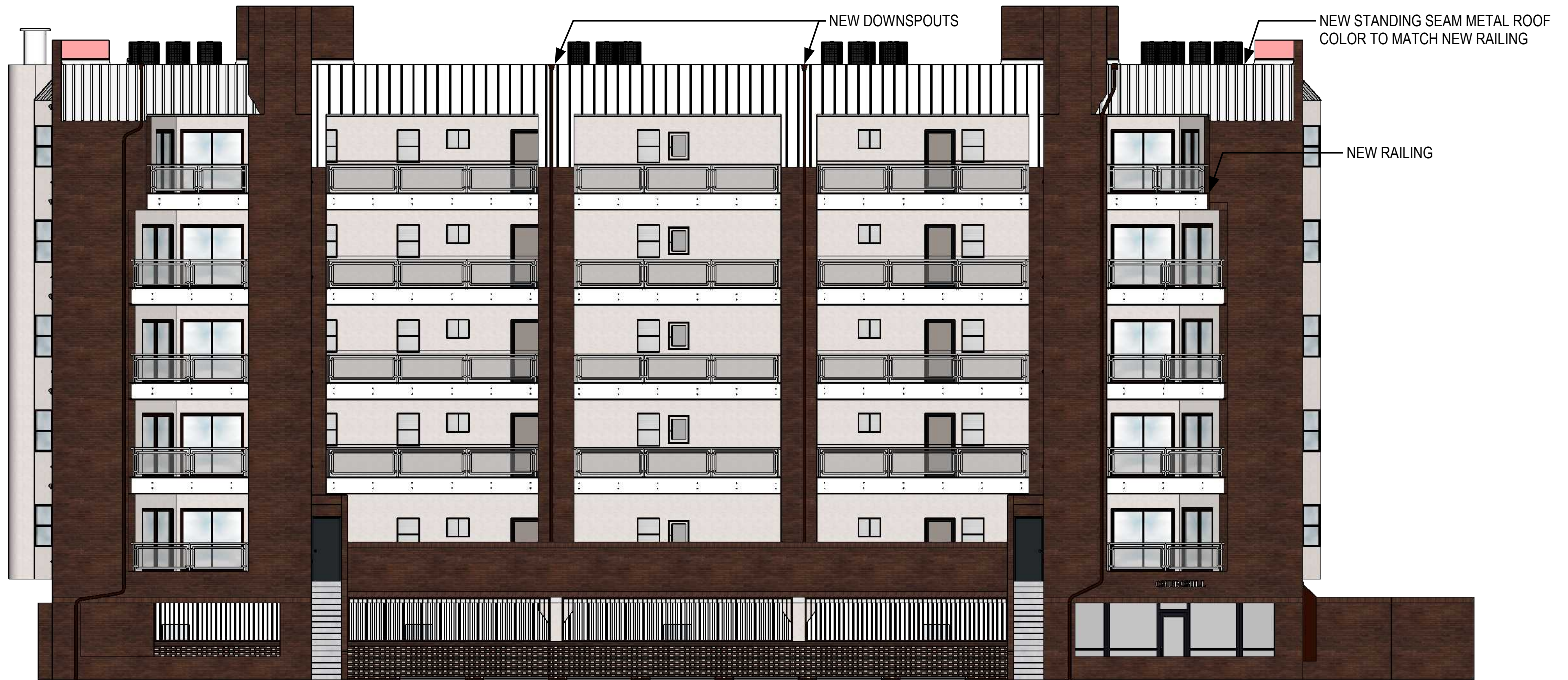
WEST ELEVATION - PROPOSED RAILING : PRIVACY RAILS
