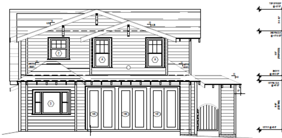
1 PROPOSED REAR ELEVATION 1/4" = 1'-0"
