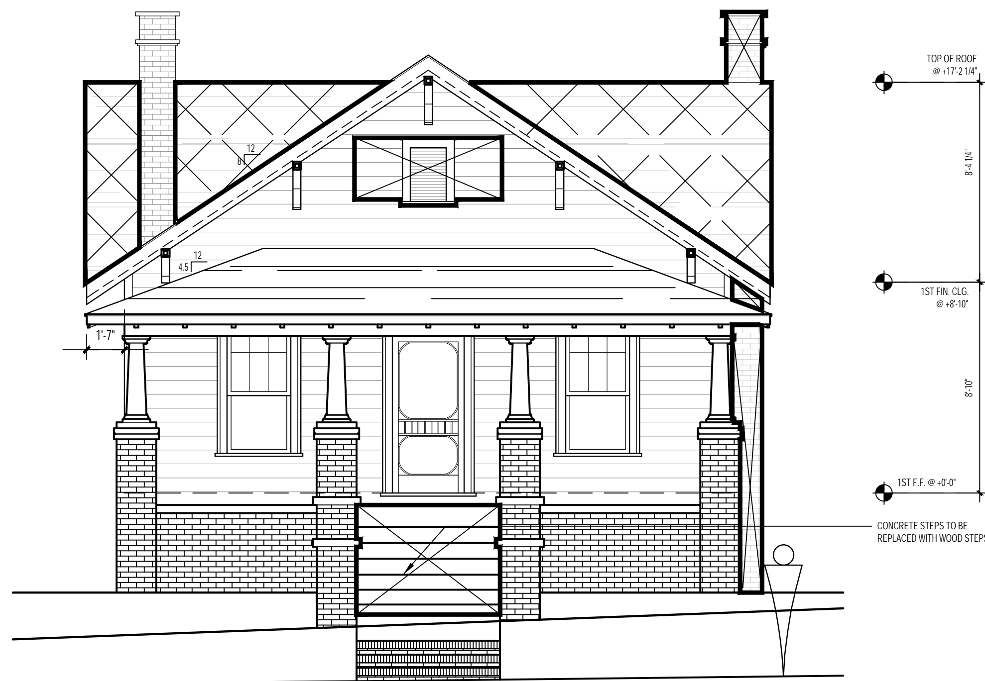
1 EXISTING FRONT ELEVATION 1/4" = 1'-0"
