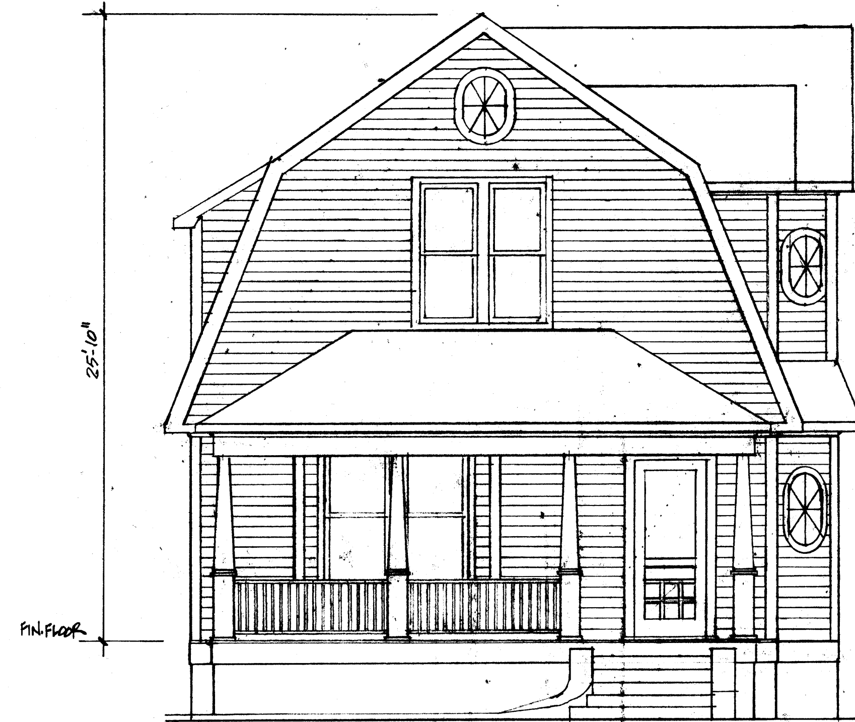
EXISTING FRONT ELEVATION (NO CHANGE IN RENOVATION) SCALE: 1/4"=1'-0"
