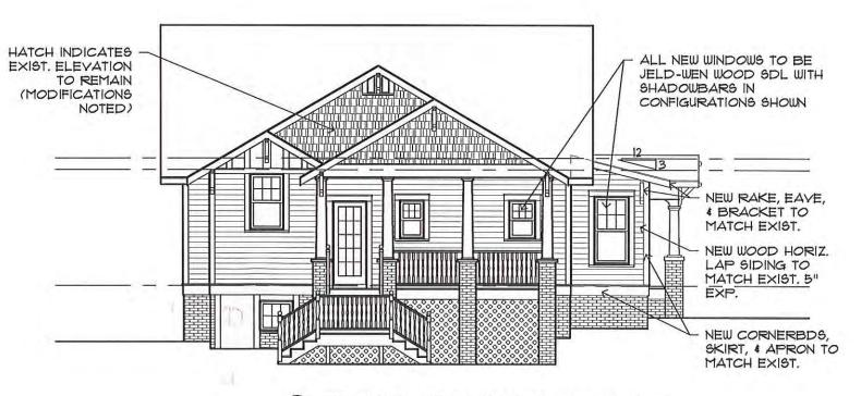
2 REAR ELEVATION (SOUTH) - PROPOSED A2.2 SCALE: 1/8"=1'-0"
