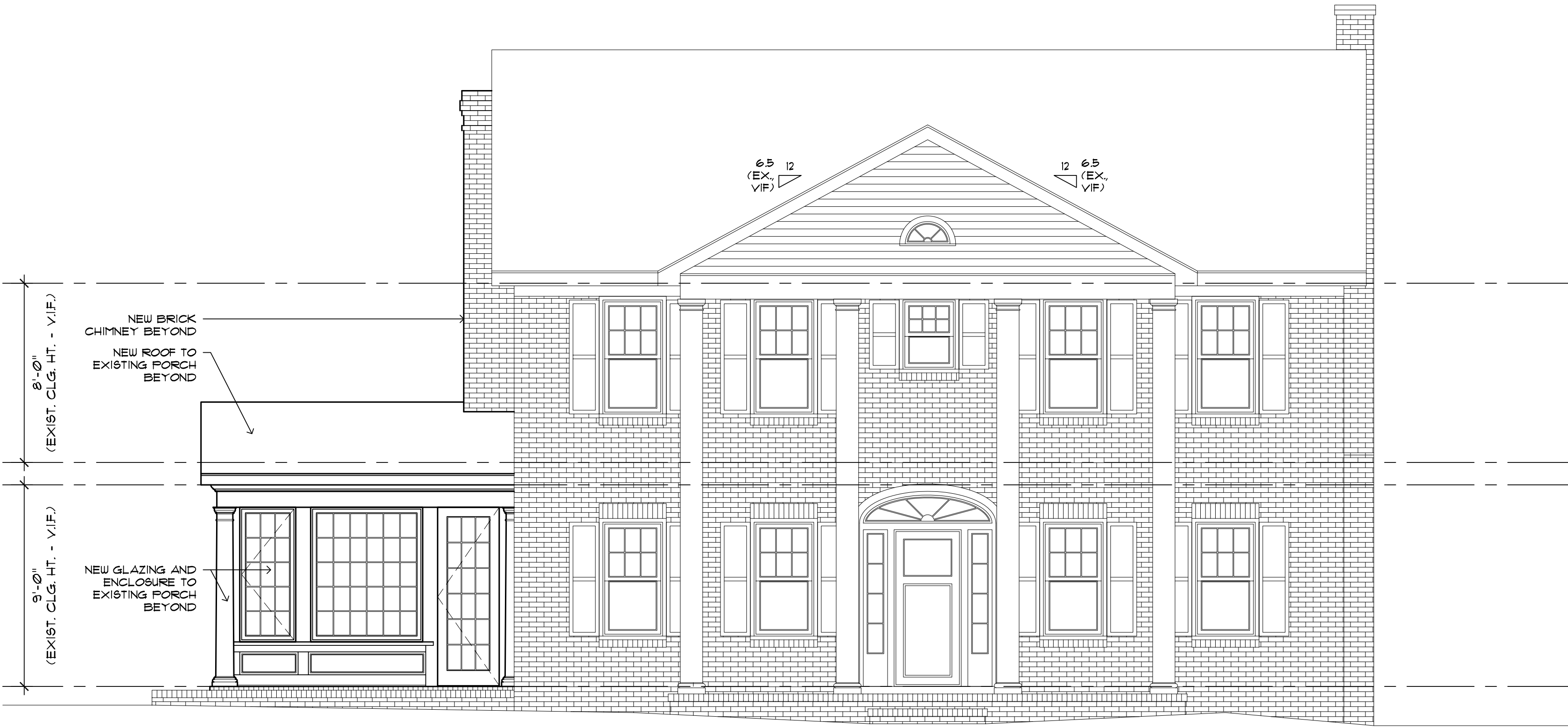
1 FRONT (NORTH) ELEVATION - MT. VERNON AVENUE A2.0 SCALE: 1/4" = 1'-0"
