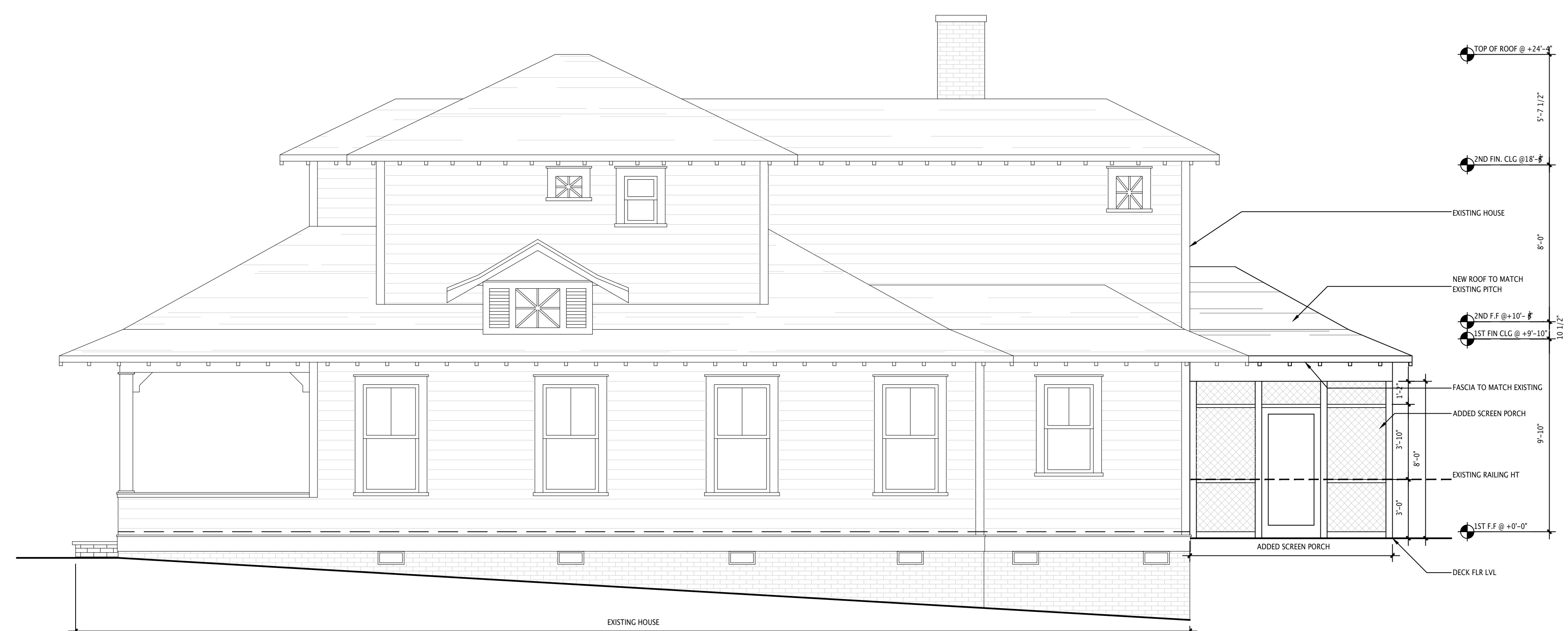
① PROPOSED RIGHT SIDE ELEVATION 1/4" = 1'-0"
