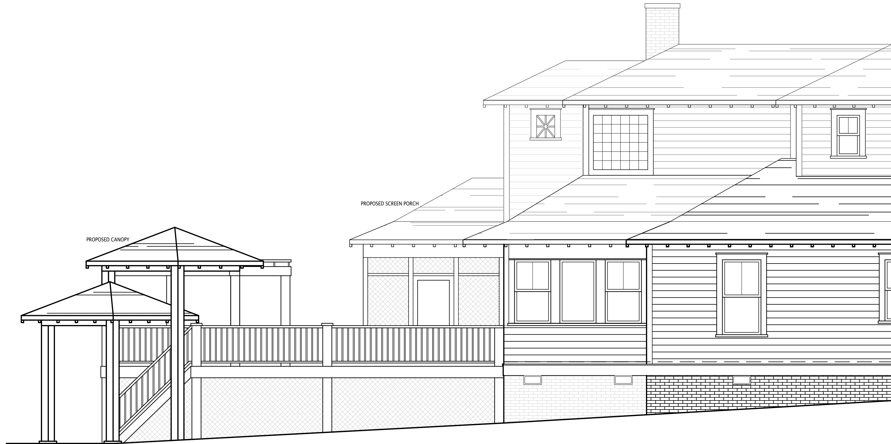
② PROPOSED PARTIAL LEFT SIDE ELEVATION 1/4" = 1'-0"
