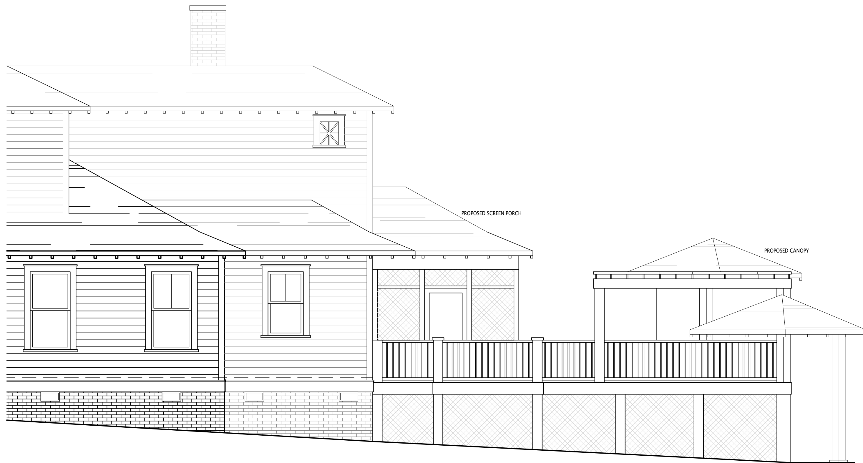
① PROPOSED PARTIAL RIGHT SIDE ELEVATION 1/4" = 1'-0"
