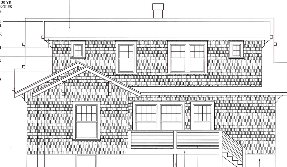
4 REAR ELEVATION - RENOVATED SCALE: 1/4" = 1'-0"
