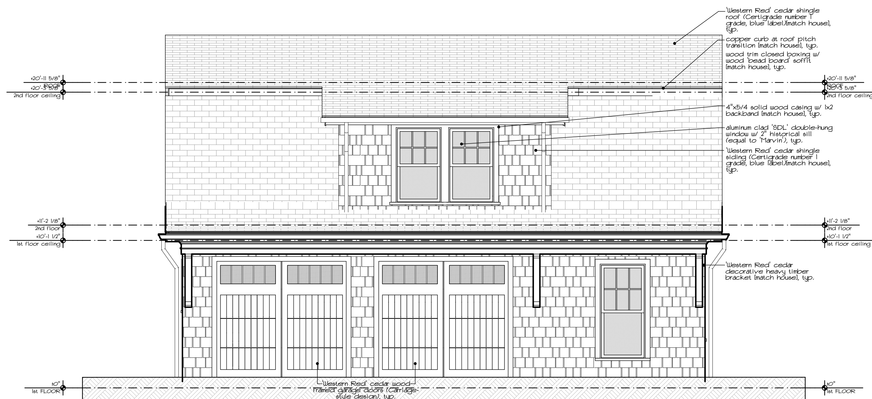
2 A2.3 Rear Elevation - Garage SCALE: 1/4" = 1'-0"
