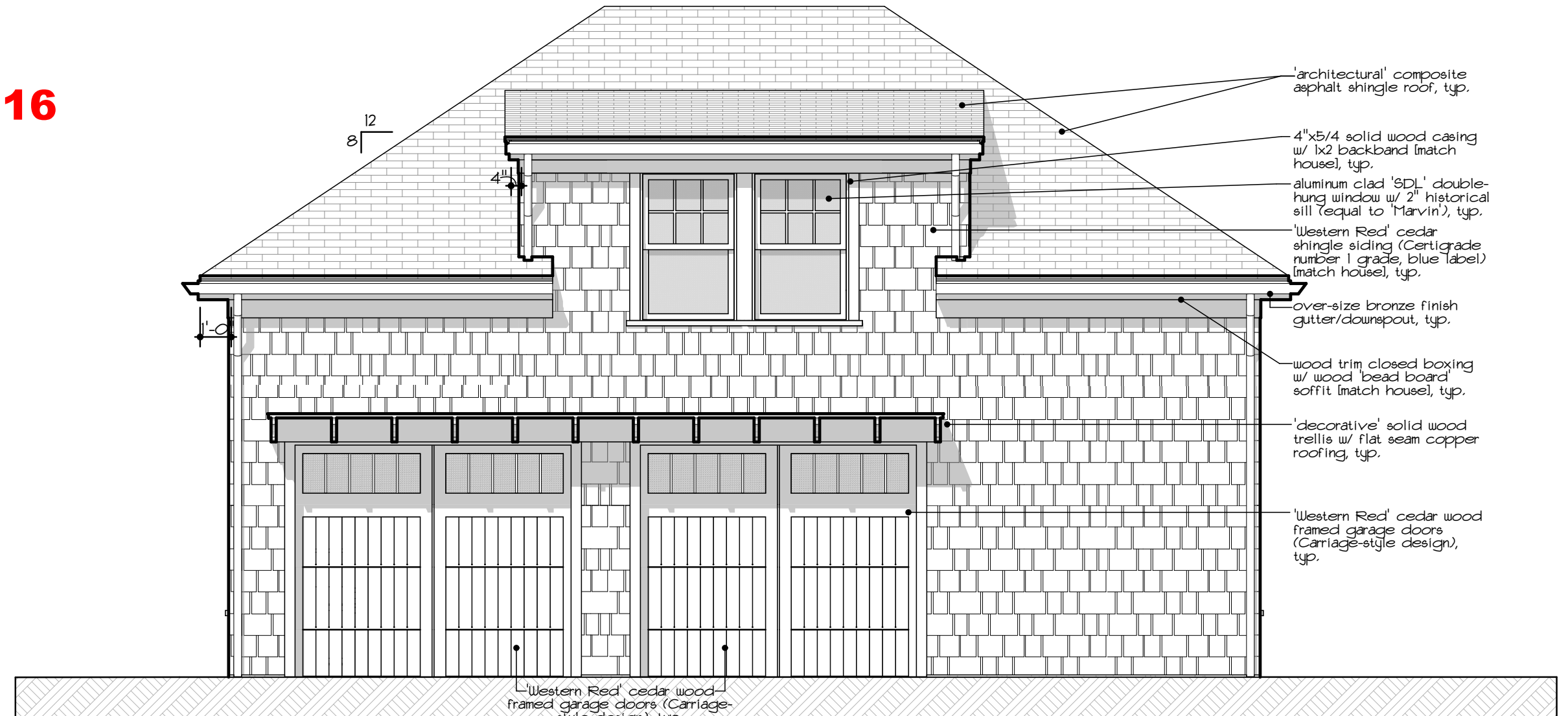
2 Rear Elevation - Garage SCALE: 1/4" = 1'-0"
