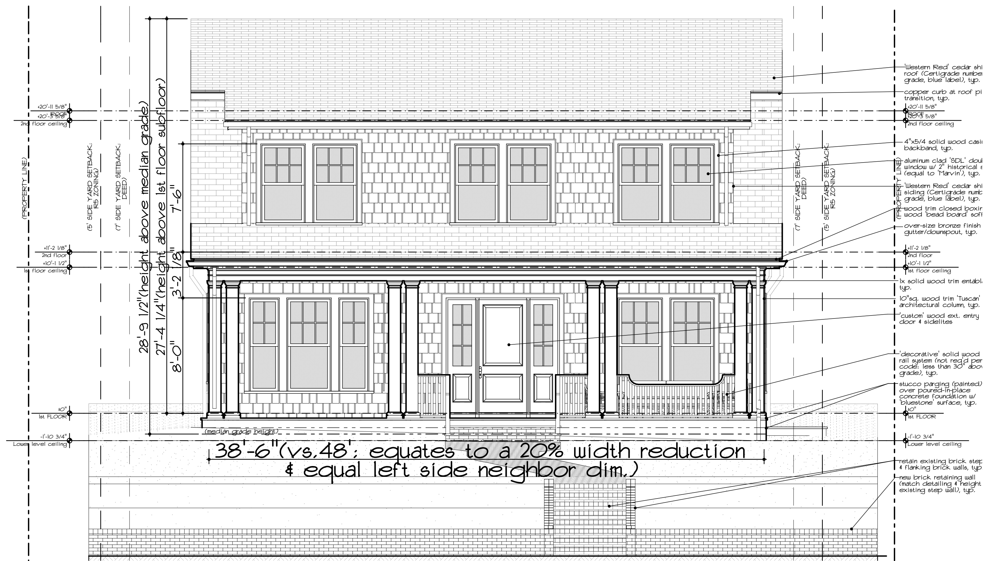
1 Front Elevation A2.1 SCALE: 1/4" = 1'-0"
