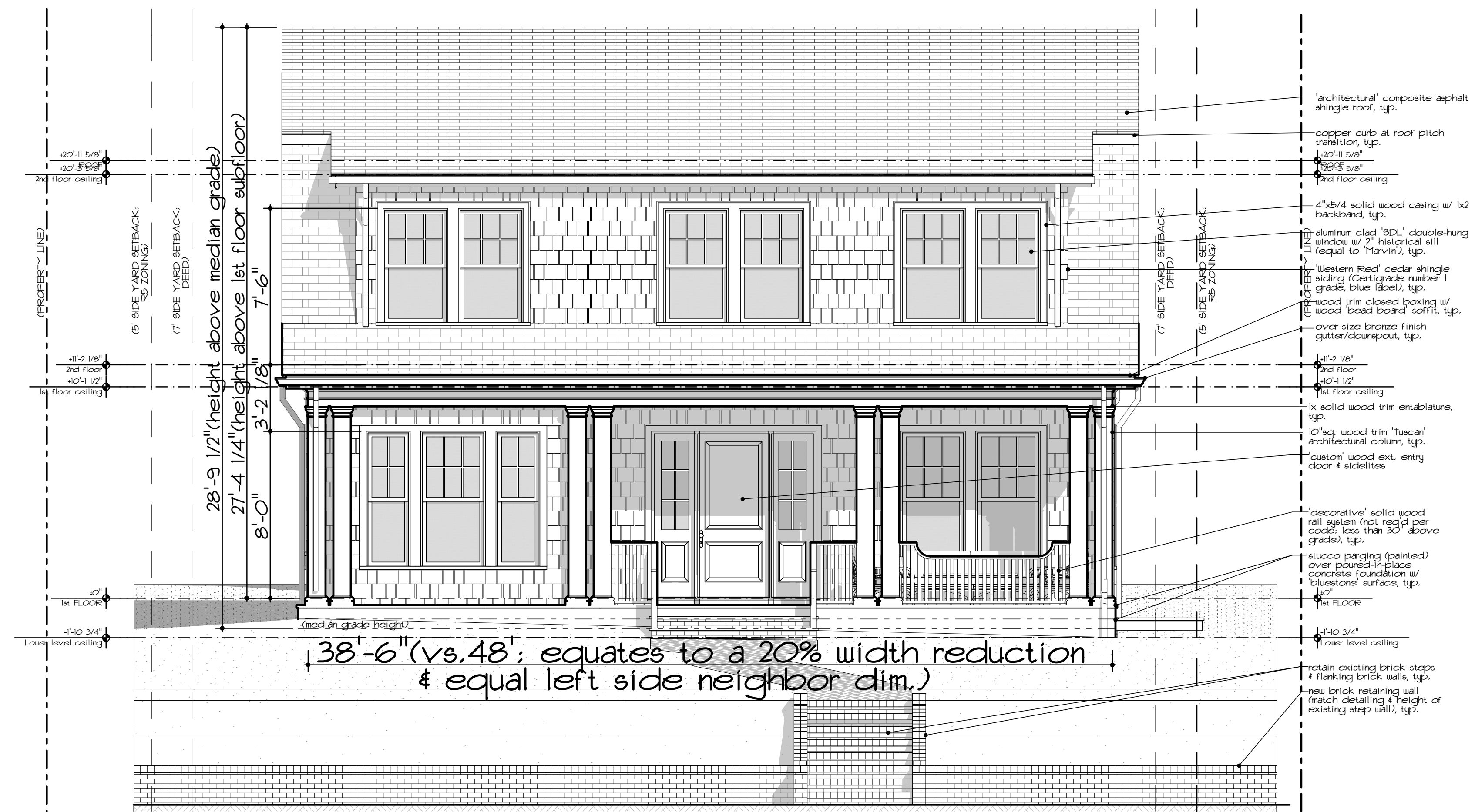
1 Front Elevation A2.1 SCALE: 1/4" = 1'-0"
