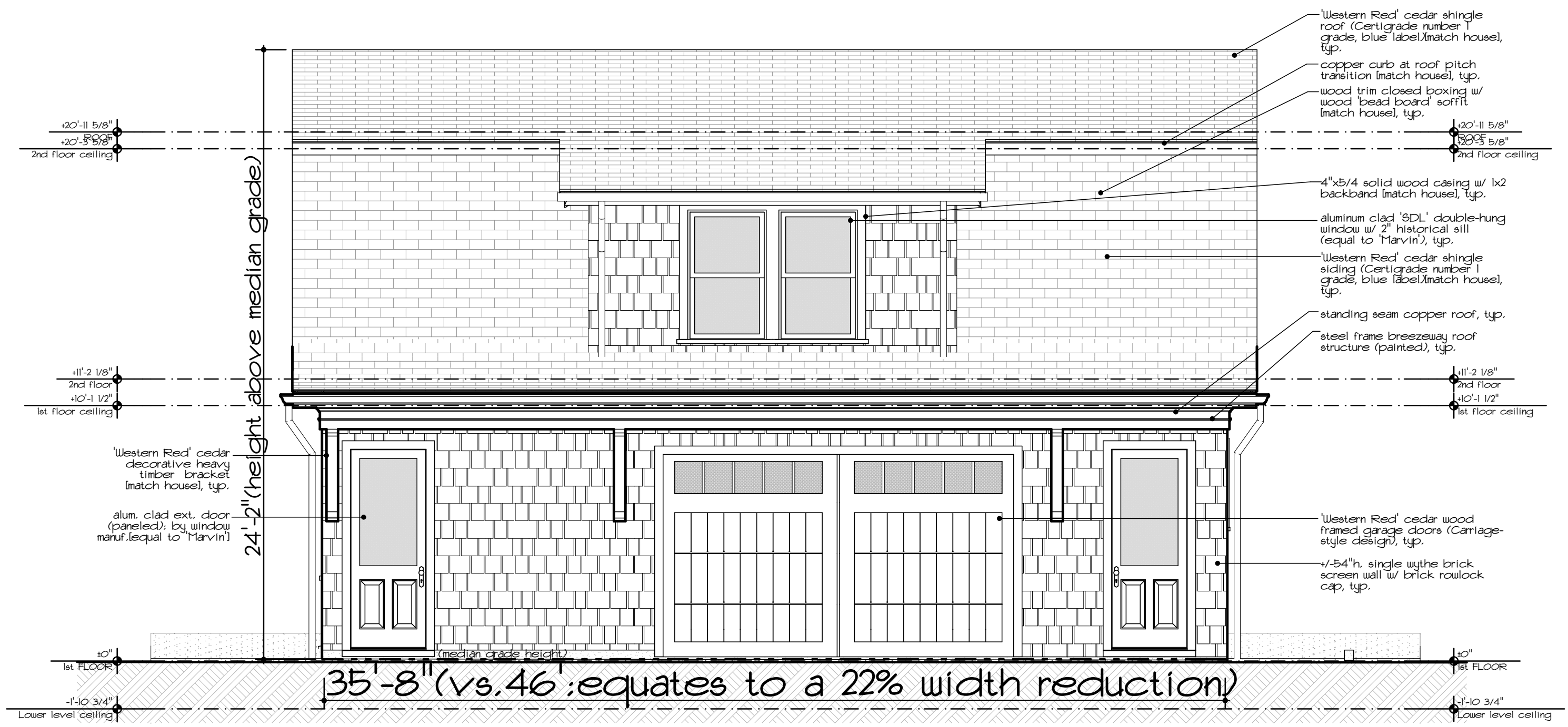
1 A2.3 Front Elevation - Garage SCALE: 1/4" = 1'-0"
