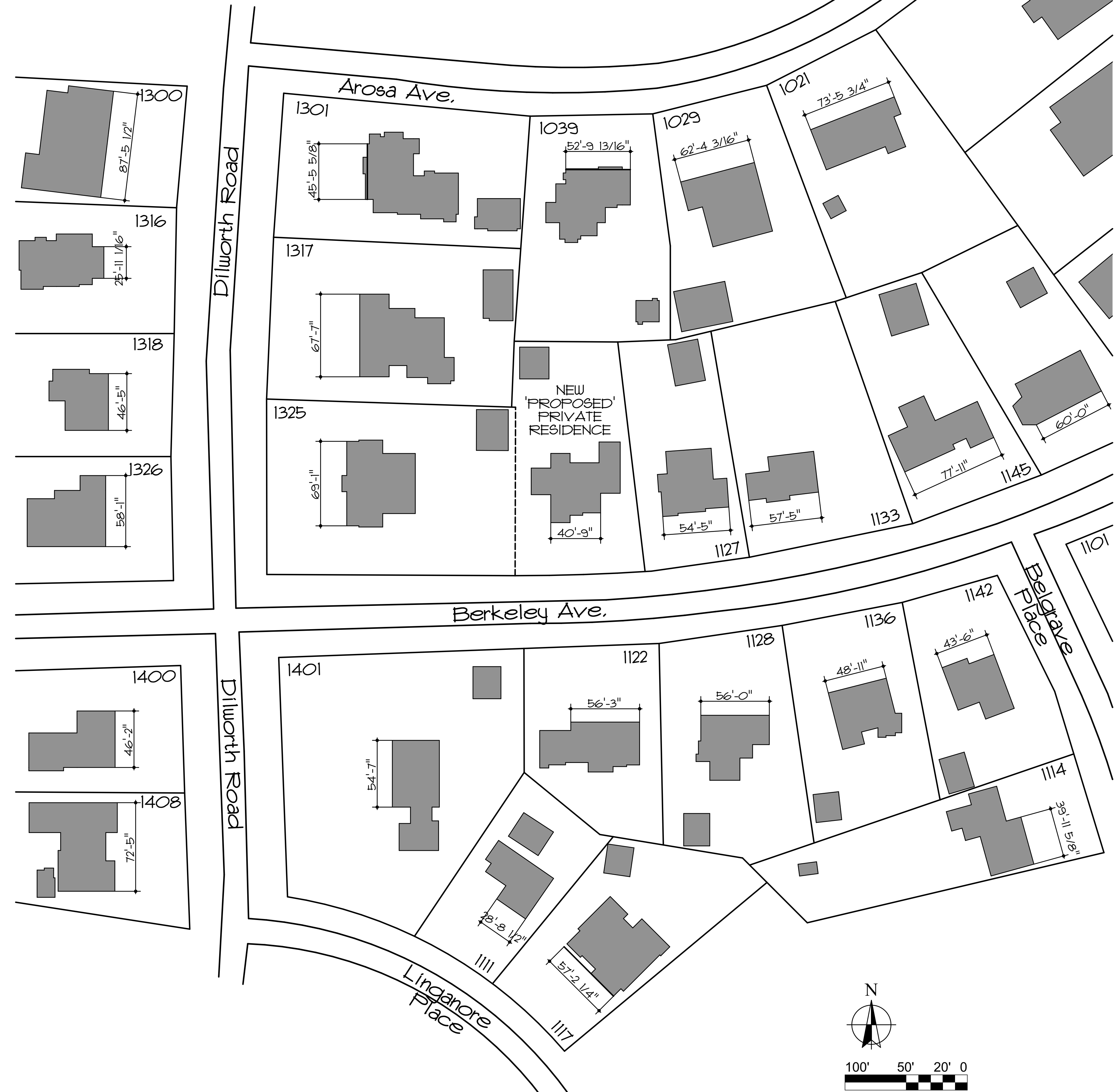
2 Plot Plan CV1.1 SCALE: 1" = 50'
