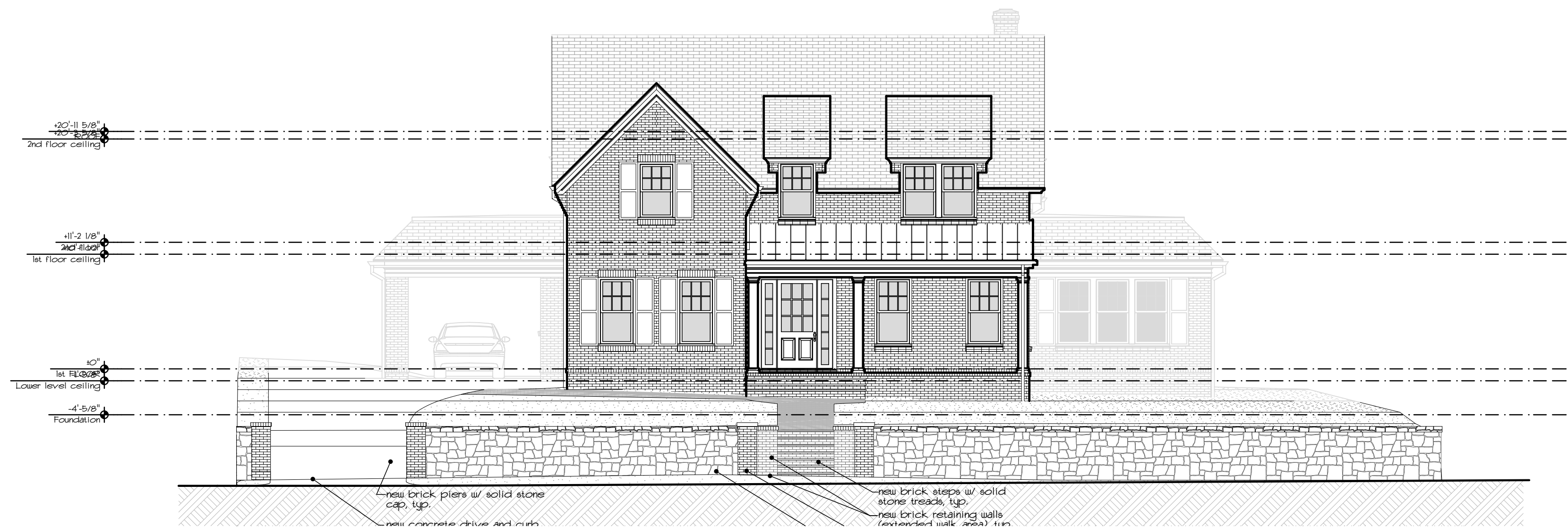
6 Front Elevation - Overall SCALE: 1/8" = 1'-0"
