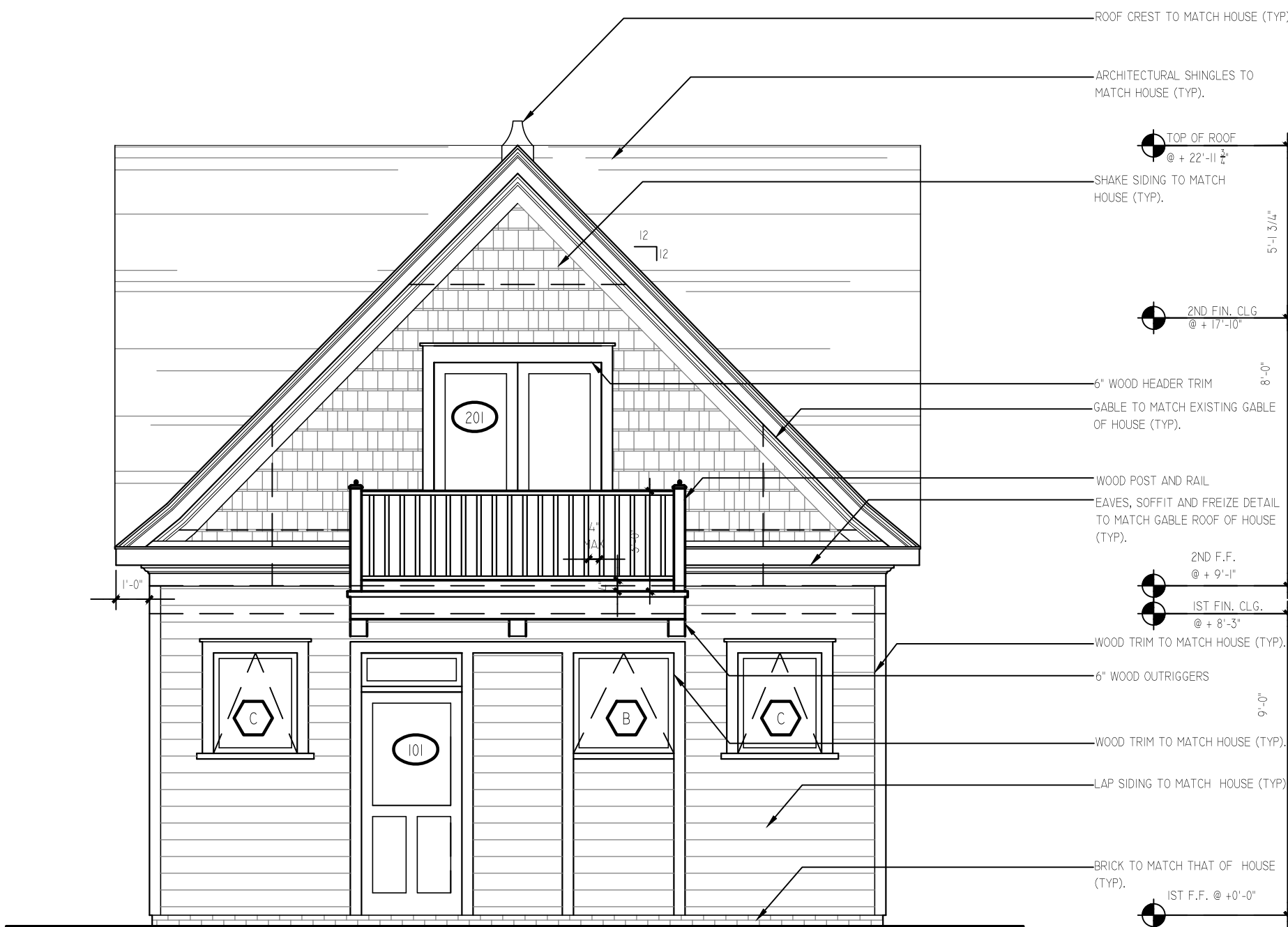
③ LEFT SIDE ELEVATION (HOUSE FACING) 1/4" = 1'-0"
