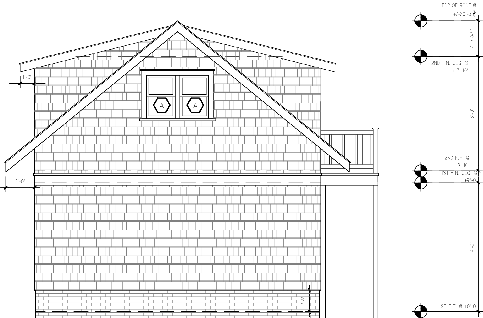
6 PROPOSED REAR ELEVATION 1/4" = 1'-0"
