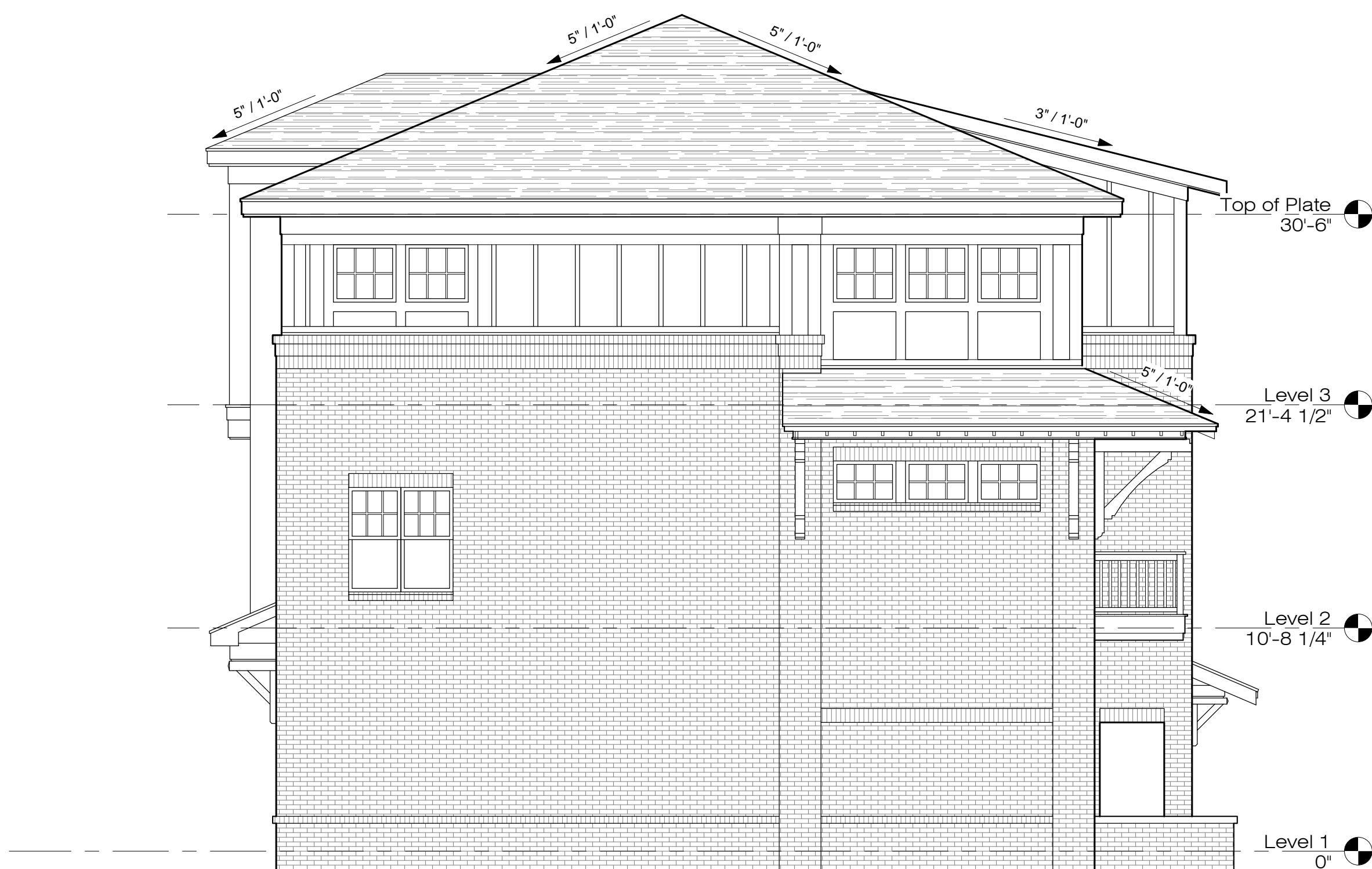
2 Building 11 - South Elevation 3/16" = 1'-0"
