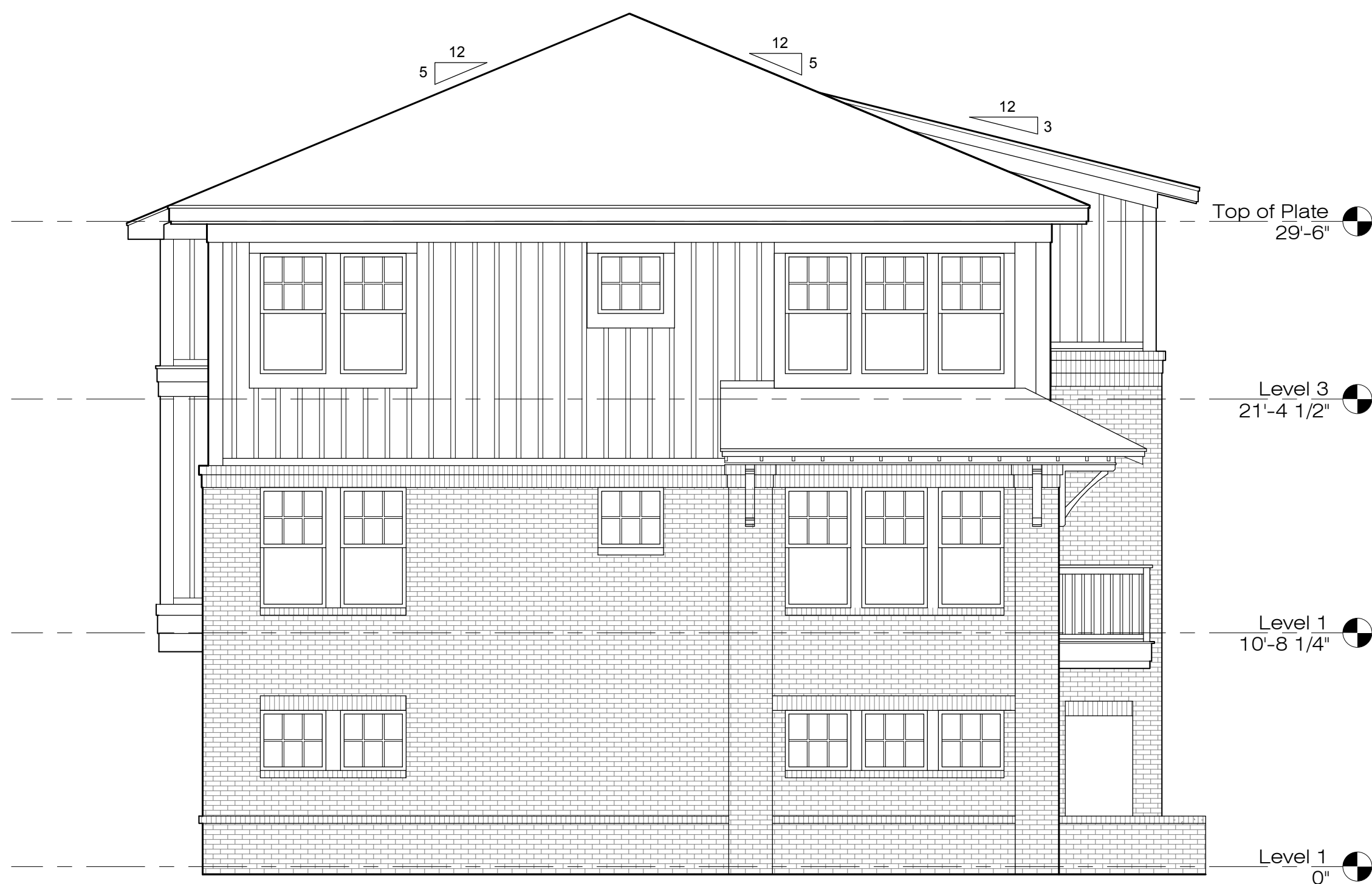
2 Building 2 North Elevation, South Mirrored (Bldg 7-10 Similar) 3/16" = 1'-0"
