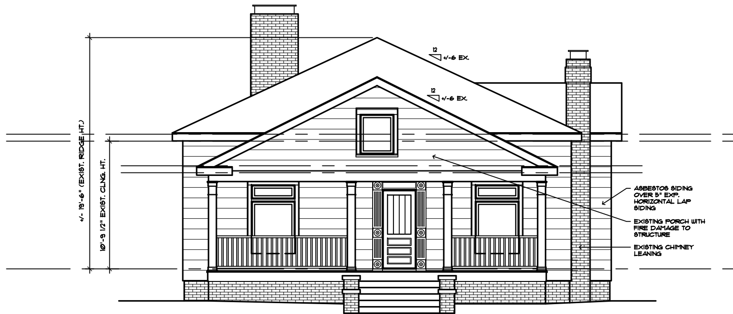
1 EXISTING FRONT ELEVATION - E. WORTHINGTON AVE. A2.0 SCALE: 1/8"=1'-0"
