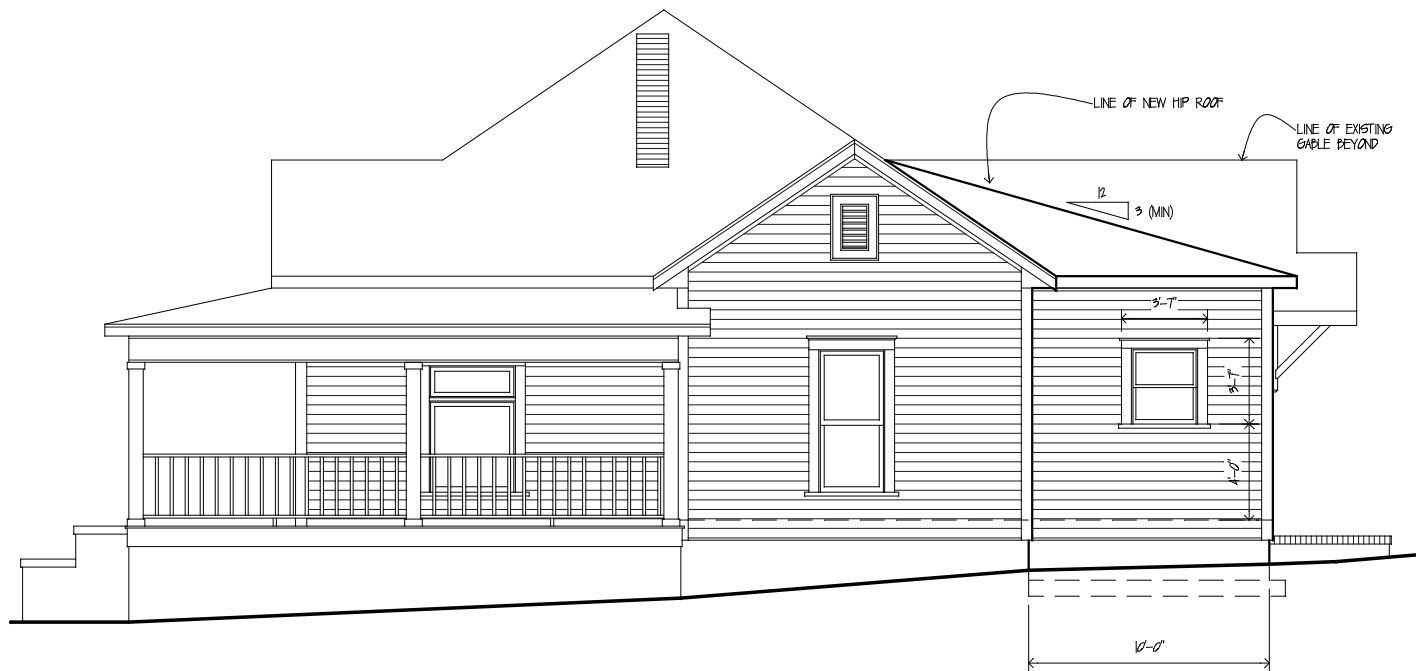
2 A-2.0 NEW RIGHT ELEVATION SCALE: 1/4" = 1'-0"
