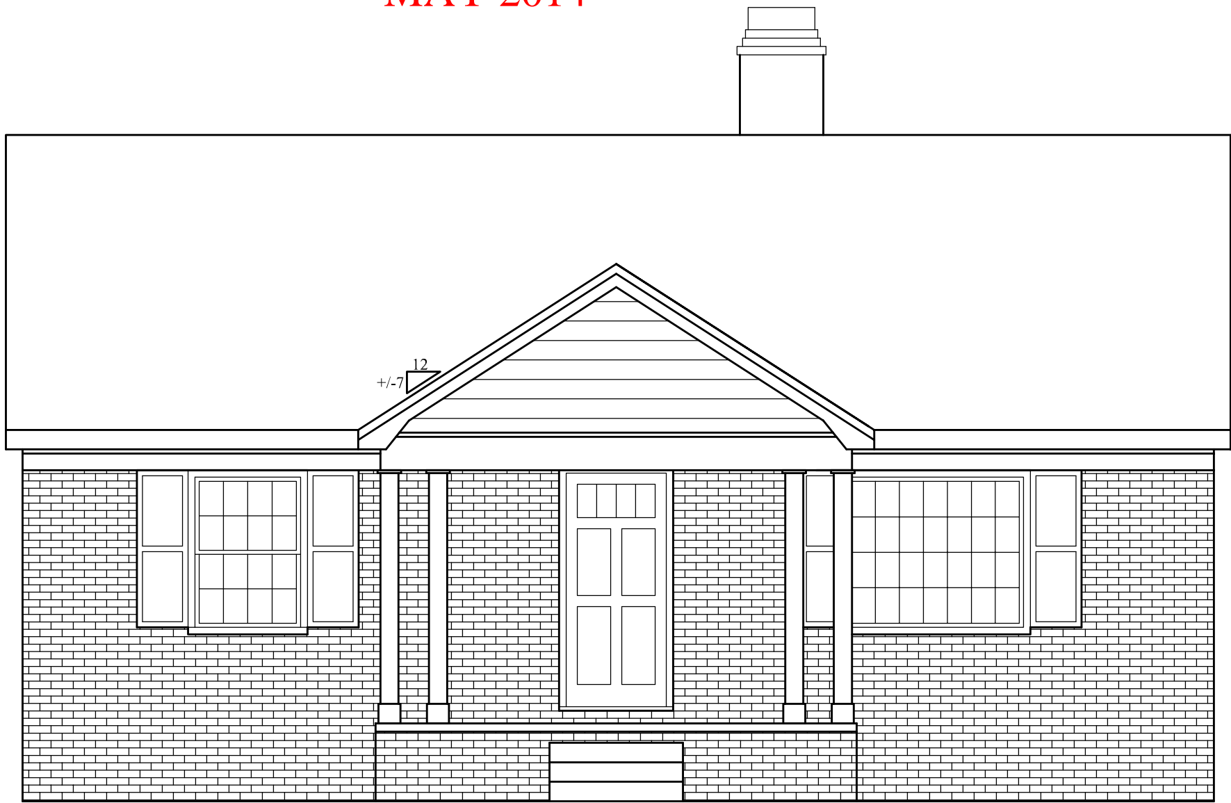
1 FRONT ELEVATION - AS BUILT A4 SCALE: 1/4" = 1'-0"
