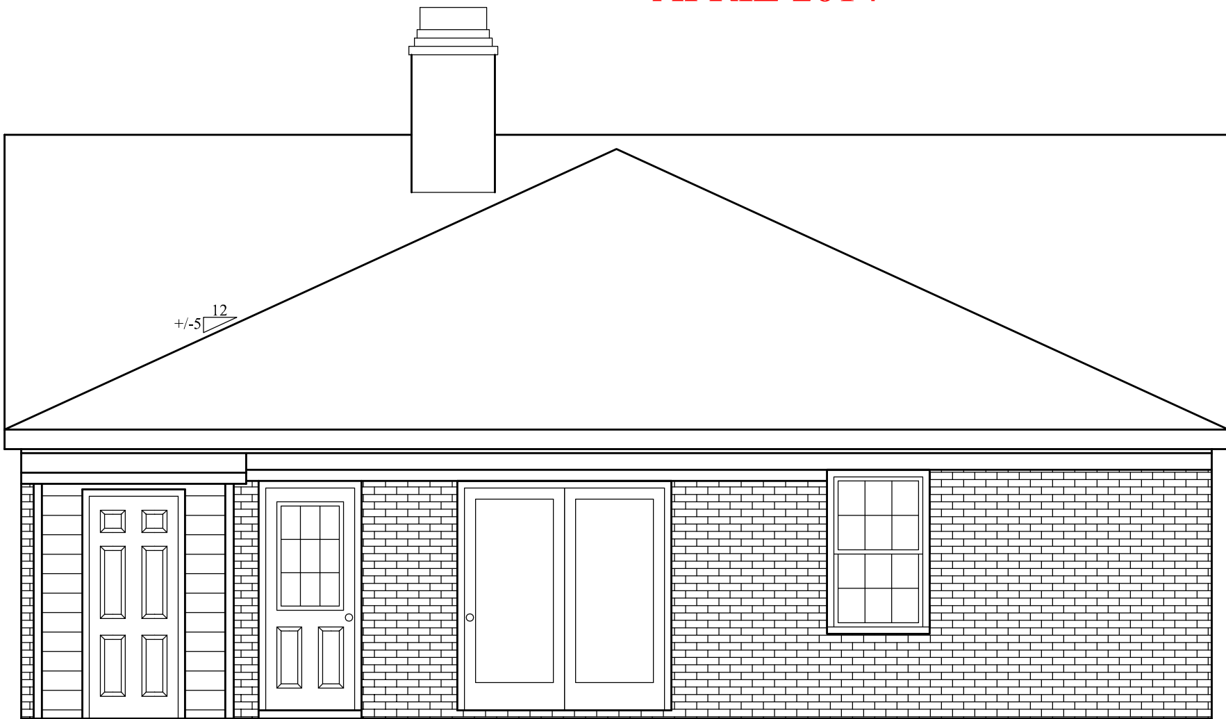
1 REAR ELEVATION - AS BUILT A6 SCALE: 1/4" = 1'-0"
