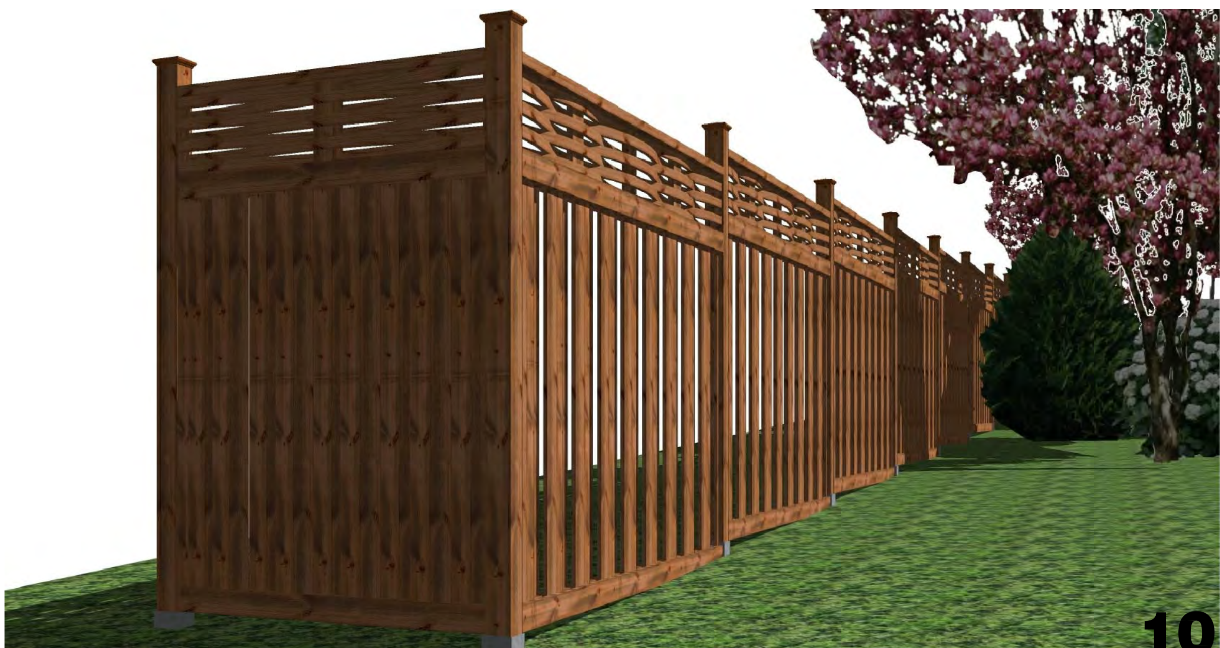
10 FENCE END PANEL VIEW of CLASS C BUFFER (Weave Alternate Shown) NTS |
