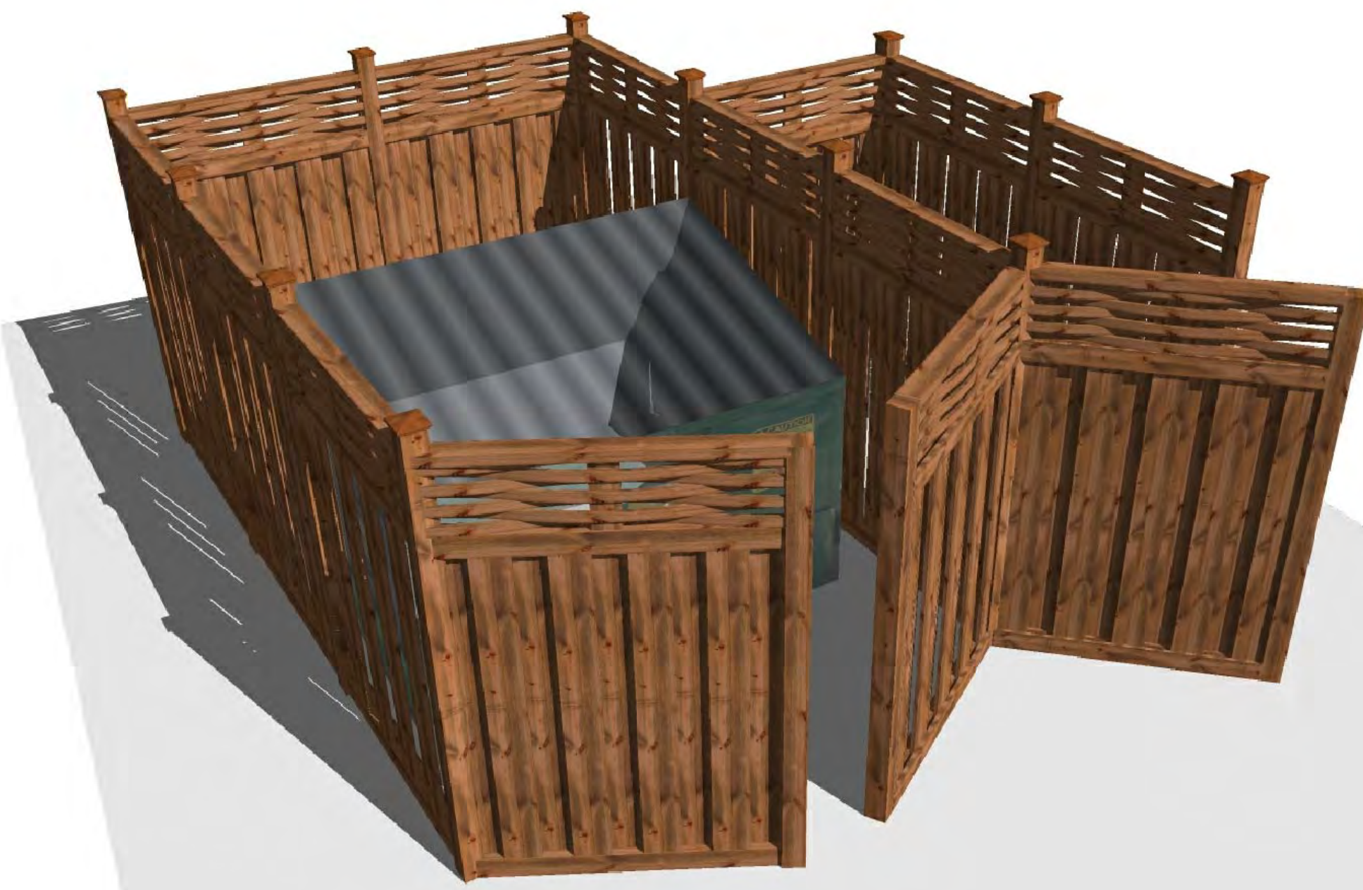
01 NTS | DUMPSTER & RECYCLING ENCLOSURE (Similar to Fence)
