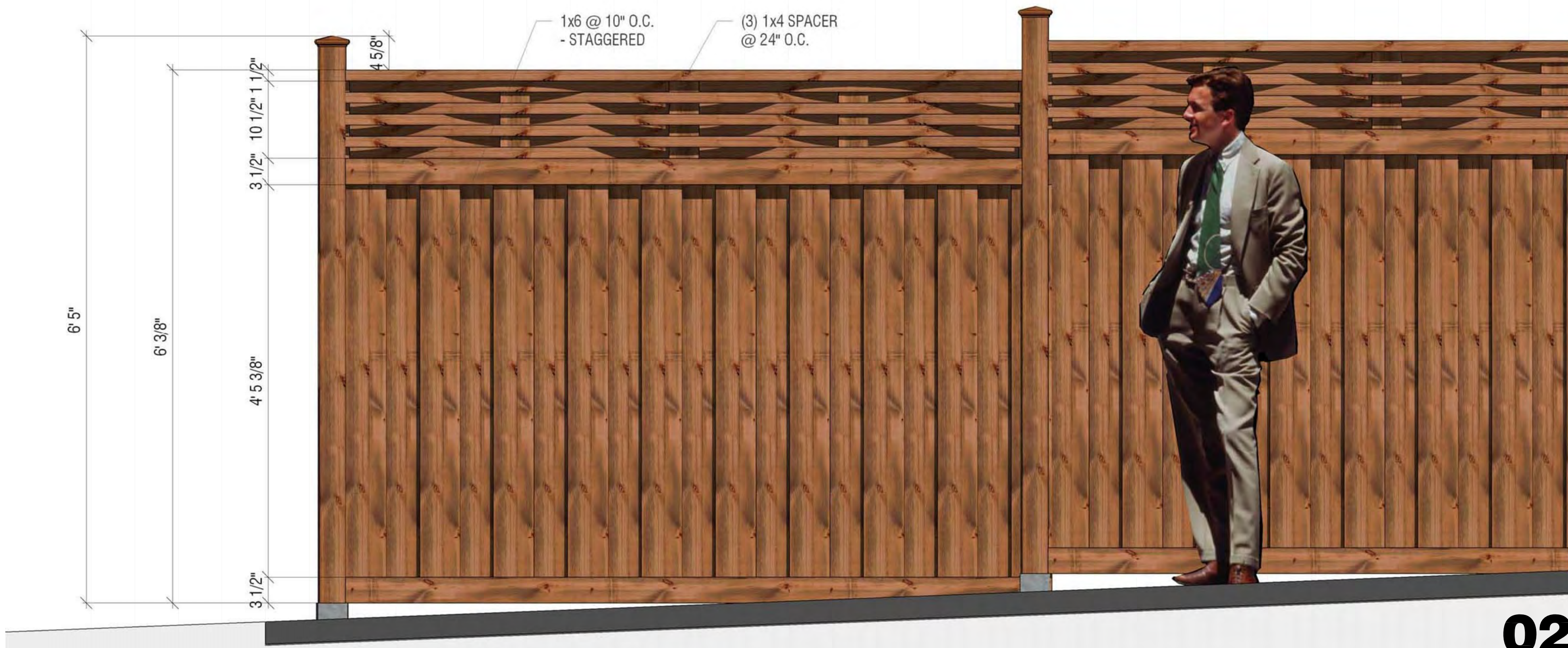
02 1" : 1'-0" | FENCE PANEL DETAIL (Weave Alternate)
