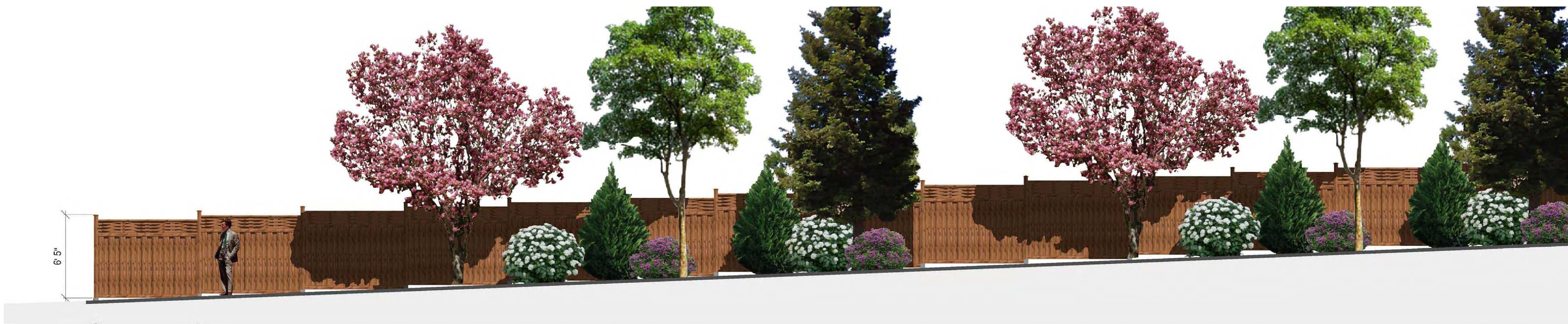
03 1/4" : 1'-0" | BUFFER FENCE ELEVATION at CLASS C BUFFER (Weave Alternate Shown -Similar Both Sides of Fence)
