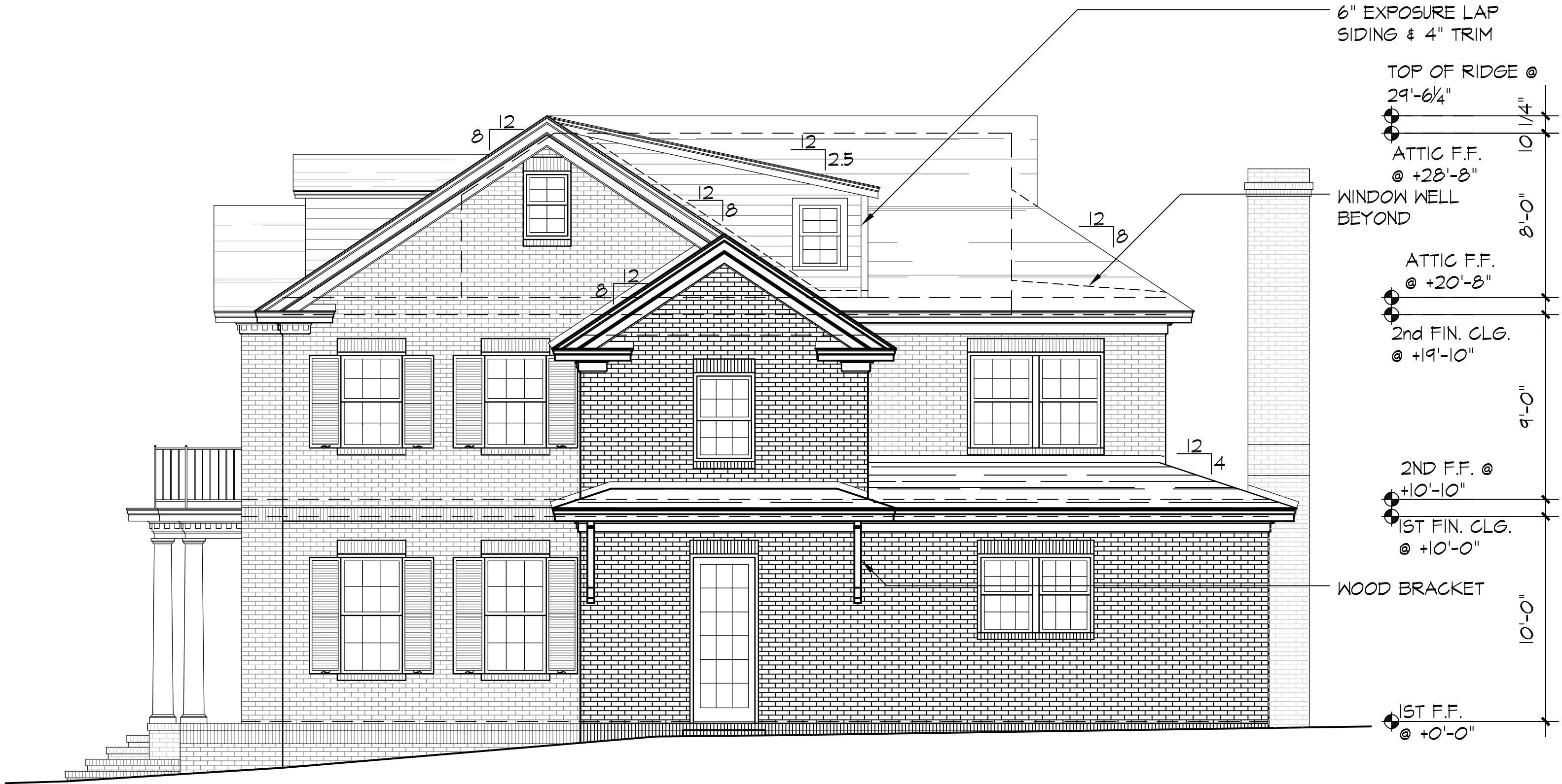
② PROPOSED RIGHT SIDE ELEVATION 1/4" = 1'-0"
