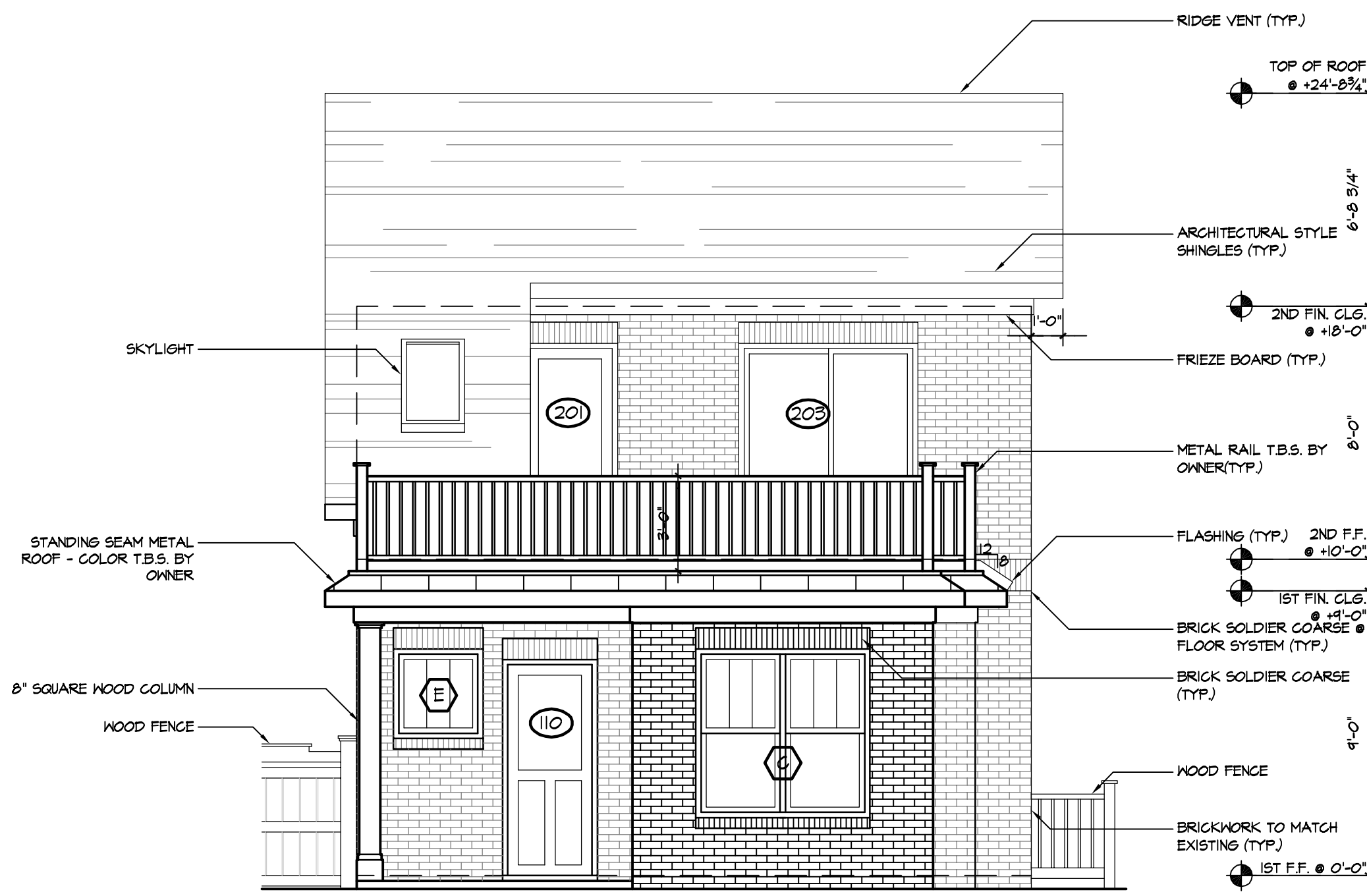
④ PROPOSED REAR ELEVATION 1/4" = 1'-0"
