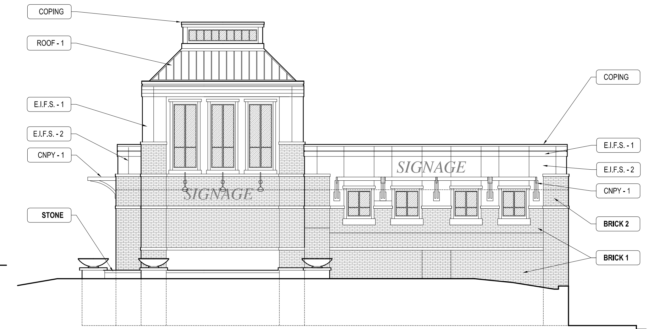
2 WEST ELEVATION REA ROAD SCALE: 1/8" = 1'-0"
