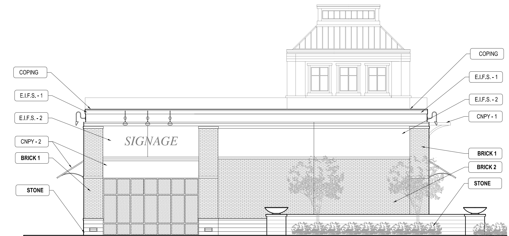
4 EAST ELEVATION AT ENTRY DRIVE SCALE: 1/8" = 1'-0"
