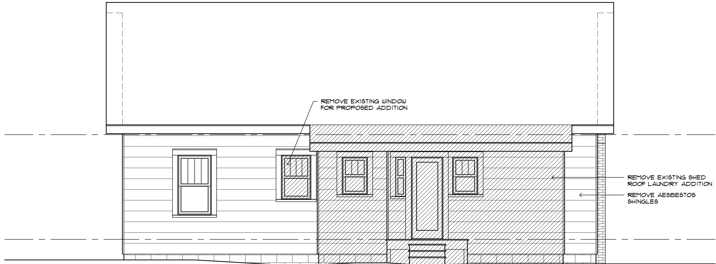
1 EXISTING REAR (SOUTH) ELEVATION A2.2 SCALE: 1/4"=1'-0"
