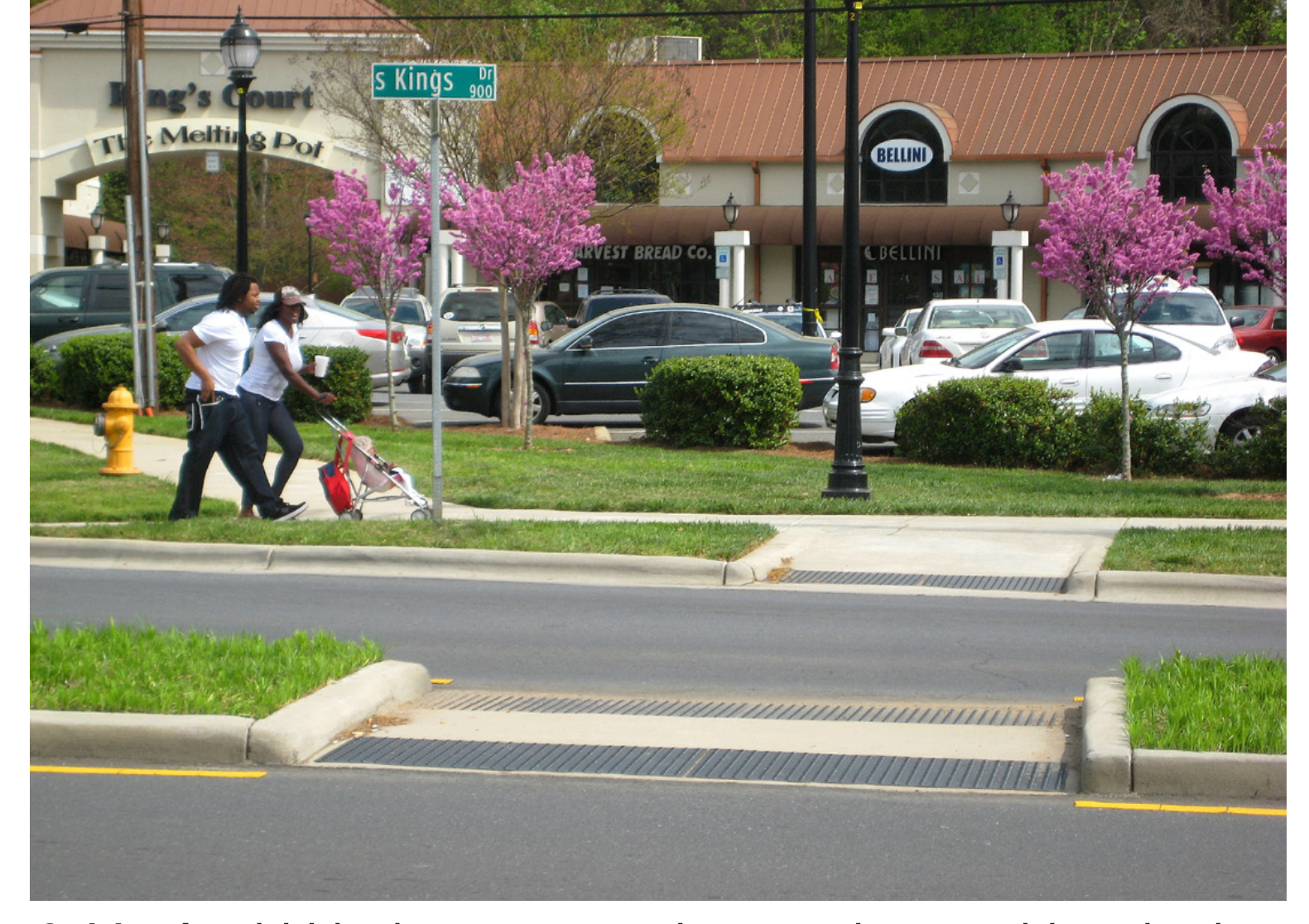
3.11 A mid-block street crossing may be considered when there is a long distance between intersections to enhance an area's walkability.
