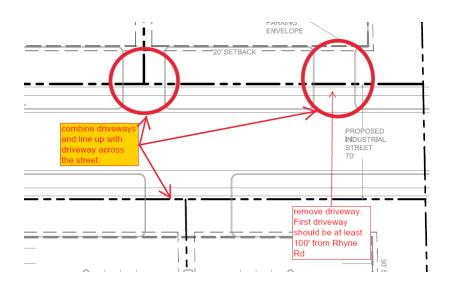
8. The petitioner should revise the site plan to eliminate the bulb out on the Proposed Industrial Street.
